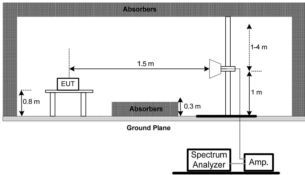
(C) For radiated emissions below 30MHz
