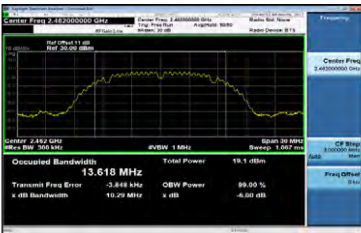
99% Band Width Test Data CH-High
