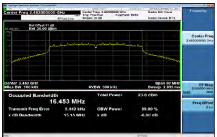
6dB Band Width Test Data CH-High
