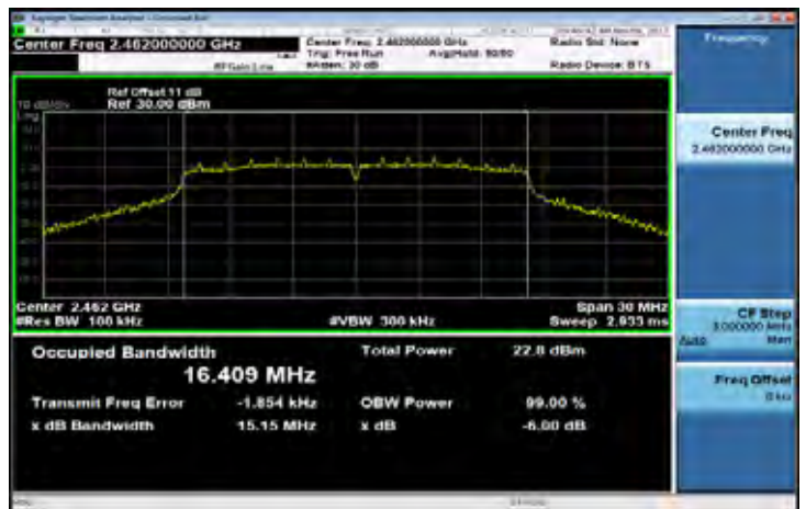
6dB Band Width Test Data CH-High
