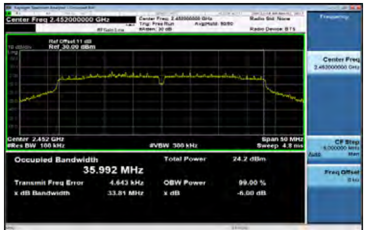
6dB Band Width Test Data CH-High
