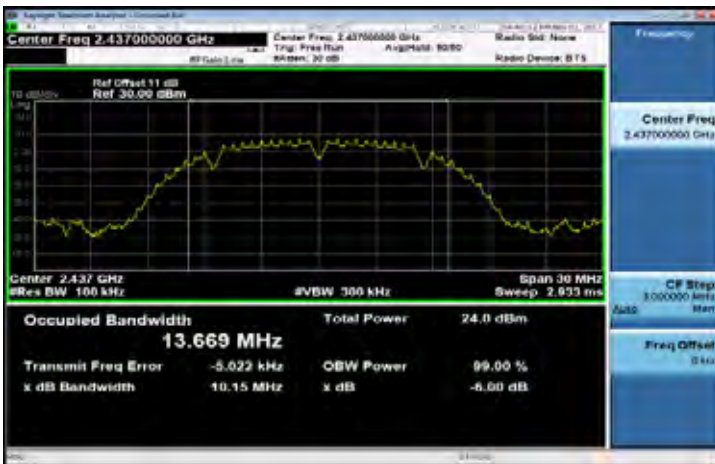
6dB Band Width Test Data CH-High
