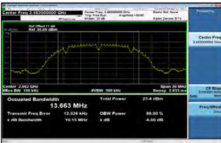
6dB Band Width Test Data CH-High
