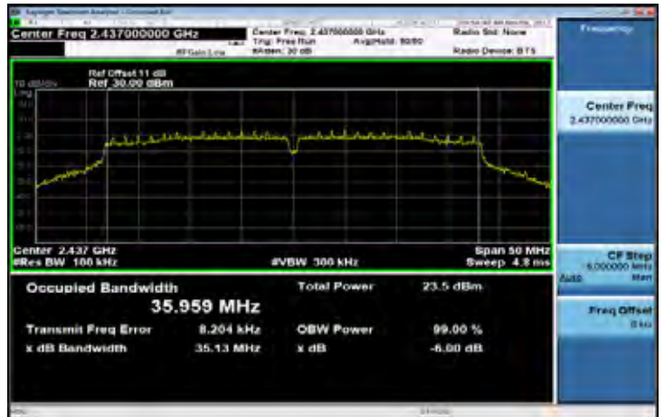
6dB Band Width Test Data CH-High
