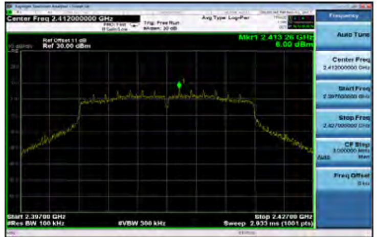
802.11n_HT20 Band Edge Limit Test Data CH-High
