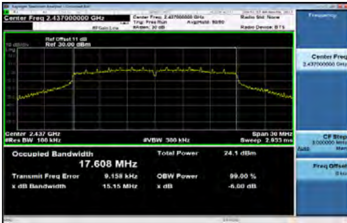
6dB Band Width Test Data CH-High
