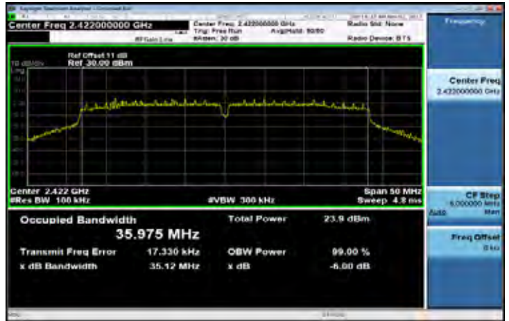
6dB Band Width Test Data CH-Mid
