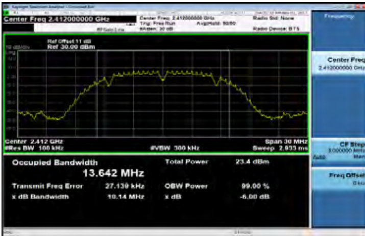
6dB Band Width Test Data CH-Mid
