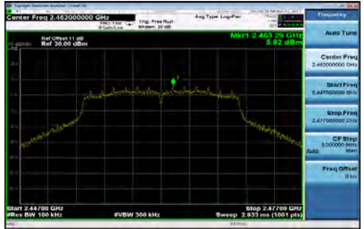
802.11n_HT20 Band Edge Limit Test Data CH-Low
