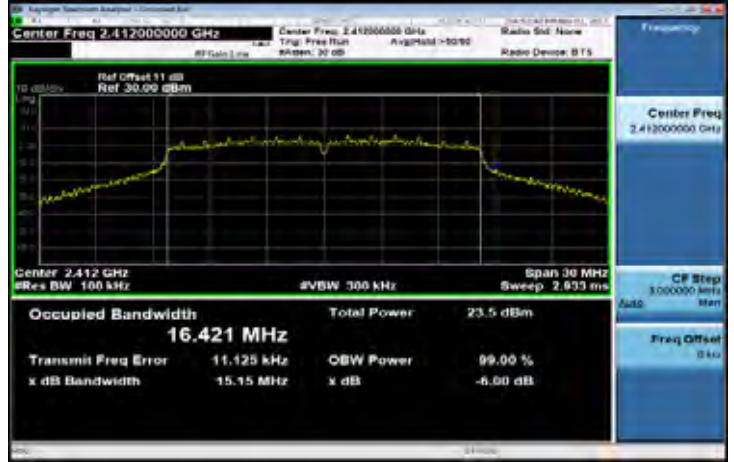
6dB Band Width Test Data CH-Mid
