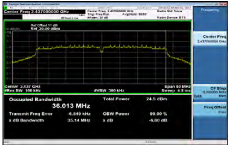
6dB Band Width Test Data CH-High
