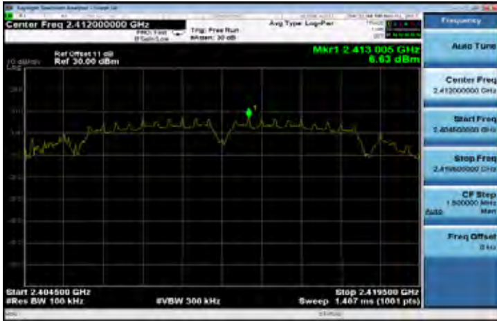
802.11b Band Edge Limit Test Data CH-High
