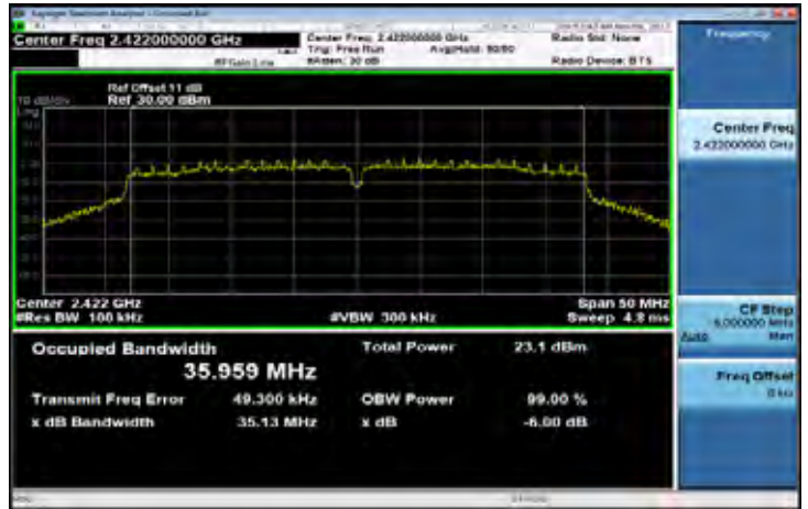
6dB Band Width Test Data CH-Mid
