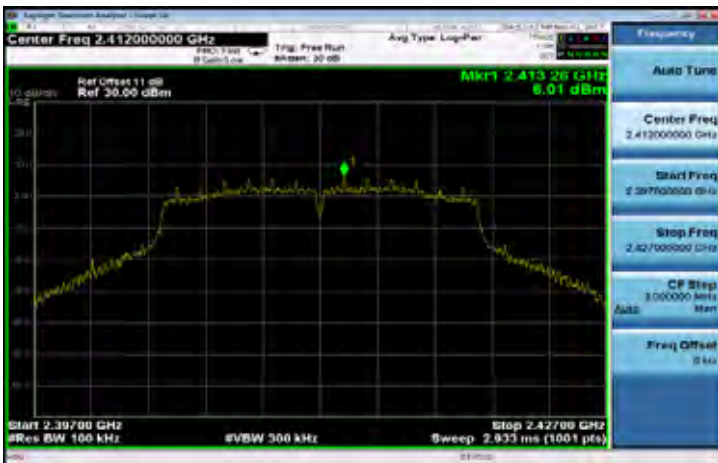
802.11g Band Edge Limit Test Data CH-Low
