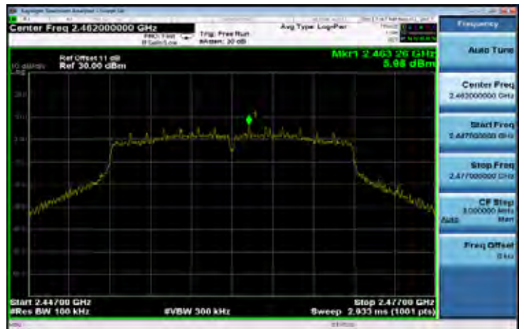
802.11n_HT20 Band Edge Limit Test Data CH-High
