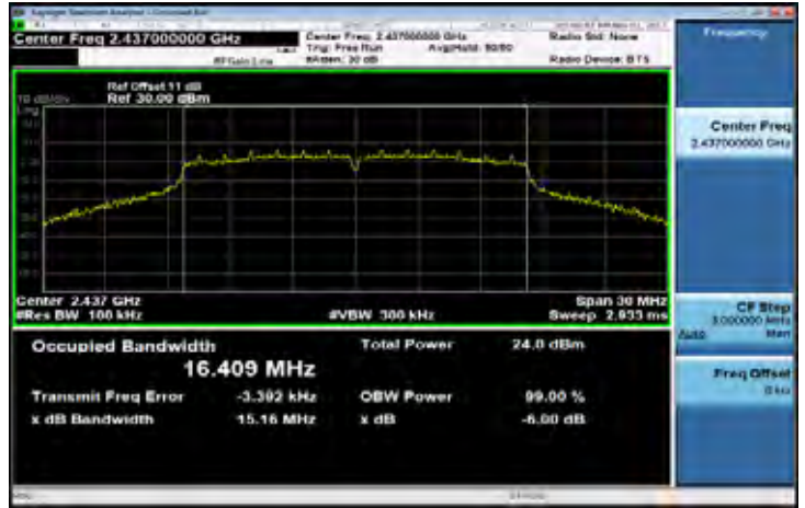
6dB Band Width Test Data CH-High
