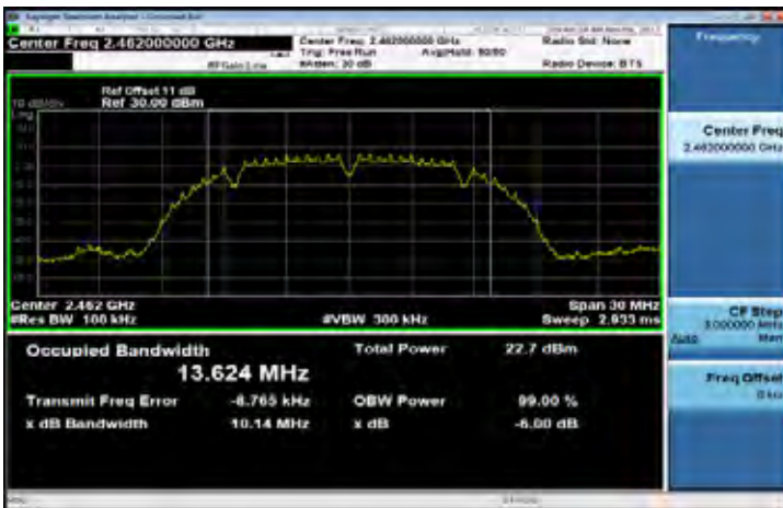
6dB Band Width Test Data CH-High
