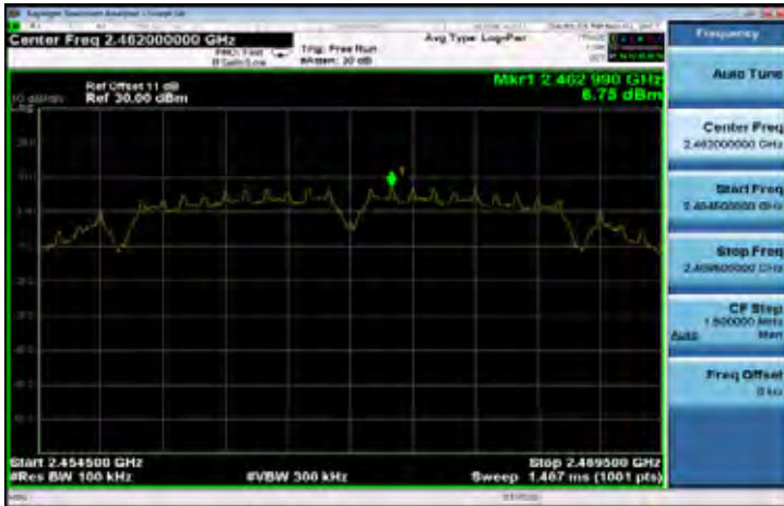
802.11g Band Edge Limit Test Data CH-Low
