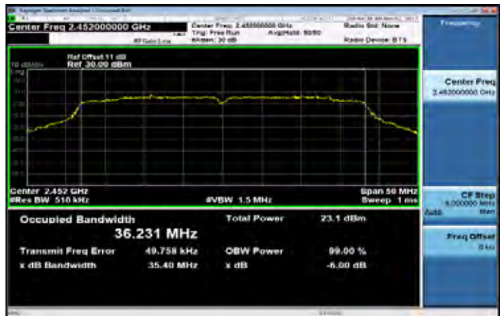
99% Band Width Test Data CH-High
