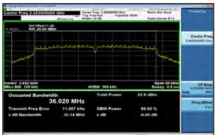
6dB Band Width Test Data CH-High
