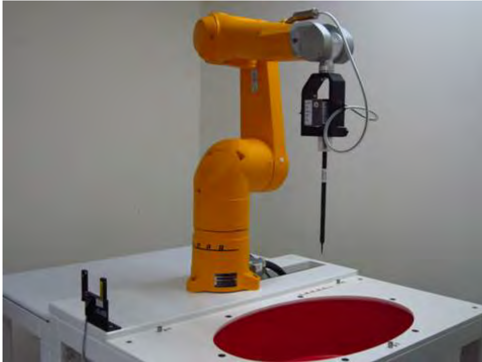
Fig.1 Photograph of the SAR measurement system
