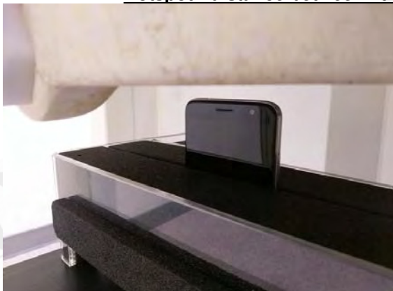
Fig.12 EUT Top side to flat phantom
