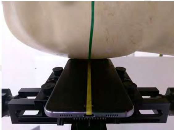
Fig.4 Right Head Section / Ear-Tilt Position(15°)
