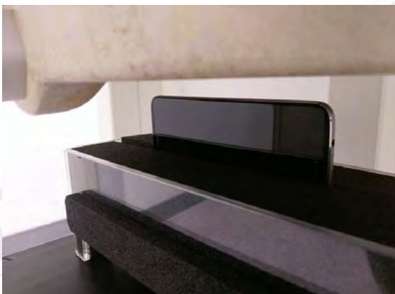
Fig.13 EUT Left side to flat phantom
