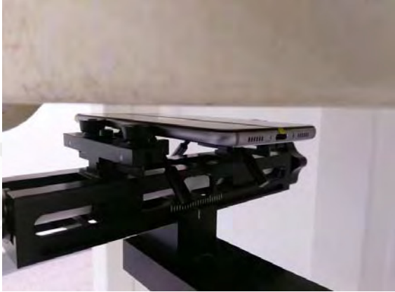
Fig.9 EUT Front side to flat phantom
