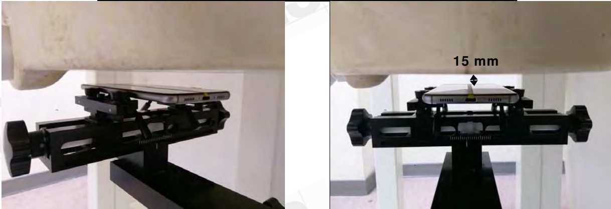
Fig.7 EUT Front side to flat phantom
