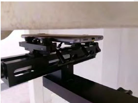
Fig.11 EUT Back side to flat phantom
