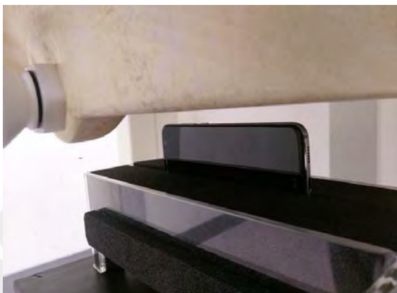
Fig.14 EUT Right side to flat phantom
