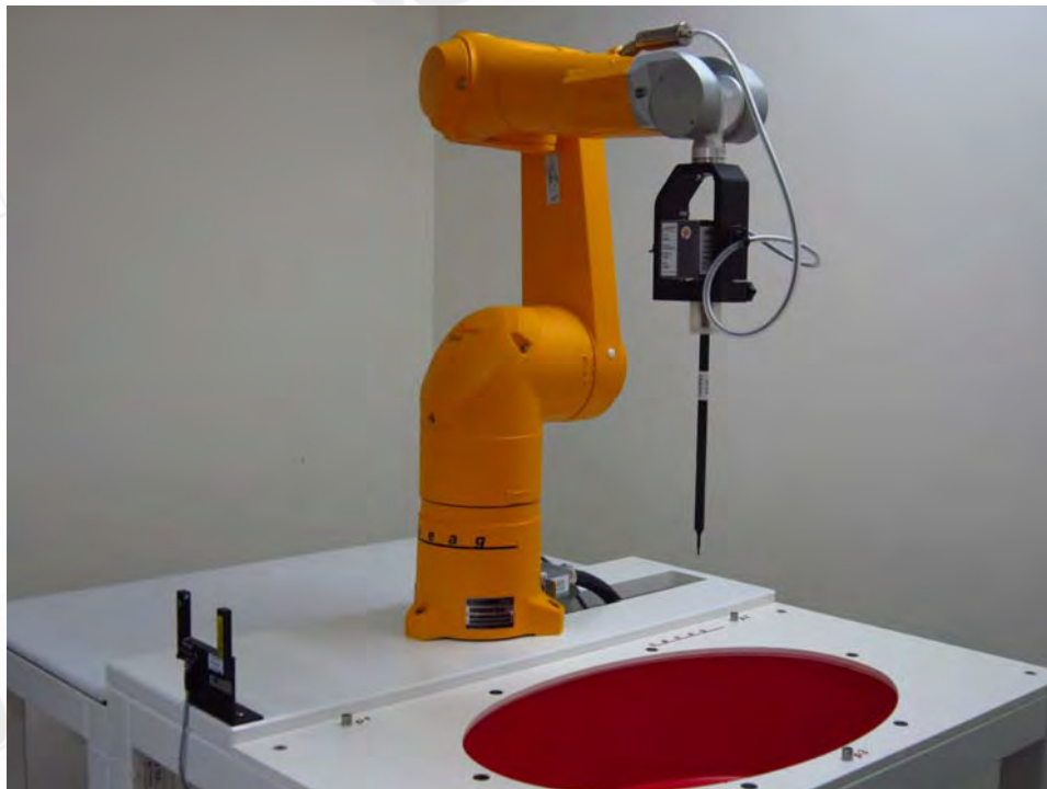
Fig.1 Photograph of the SAR measurement system
