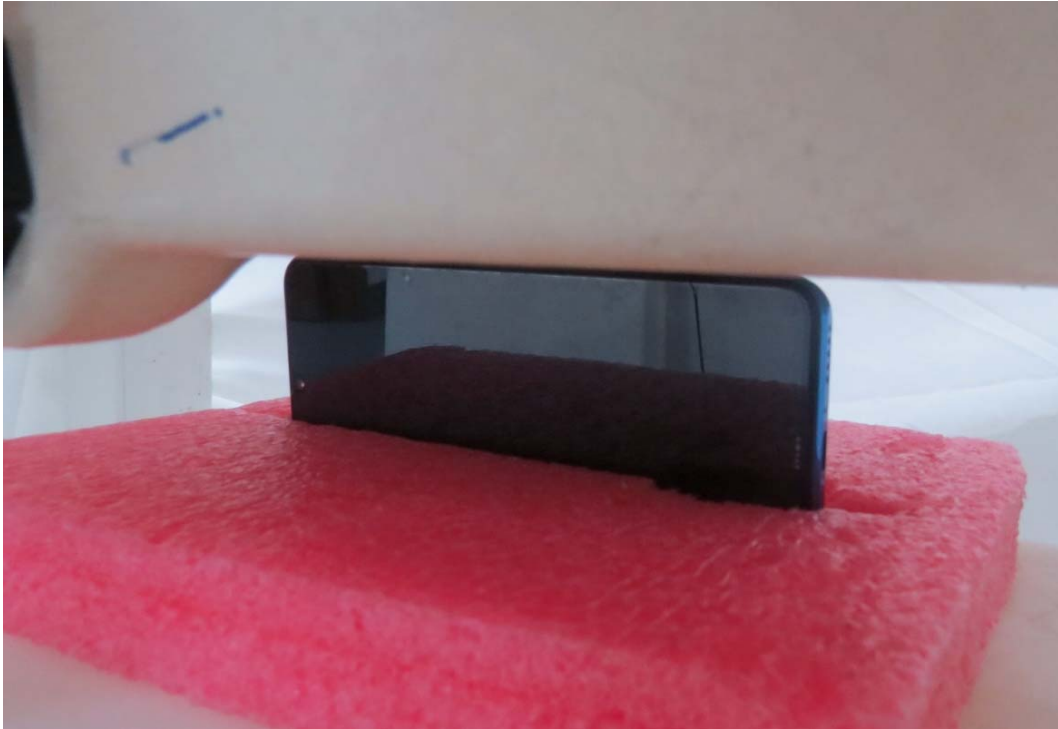
Picture 15: Right Edge, the distance from handset to the bottom of the Phantom is 0mm
