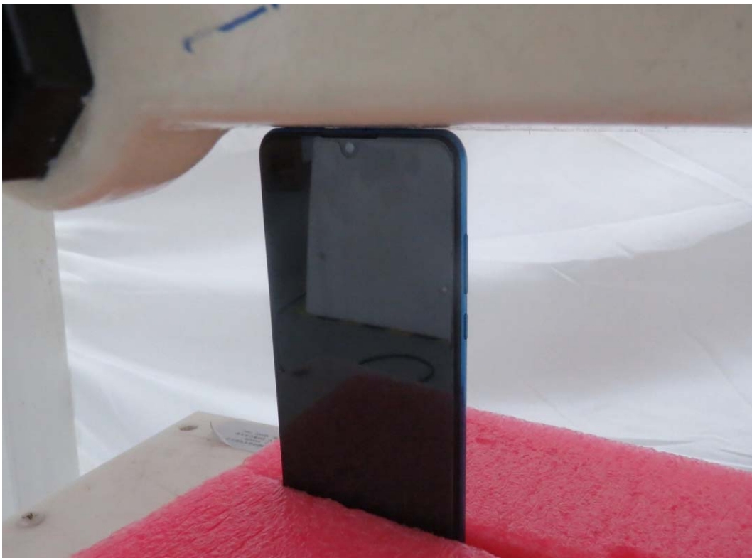
Picture 16: Top Edge, the distance from handset to the bottom of the Phantom is 0mm
