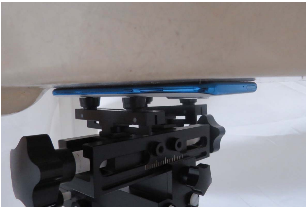
Picture 14: Front Side, the distance from handset to the bottom of the Phantom is 0mm
