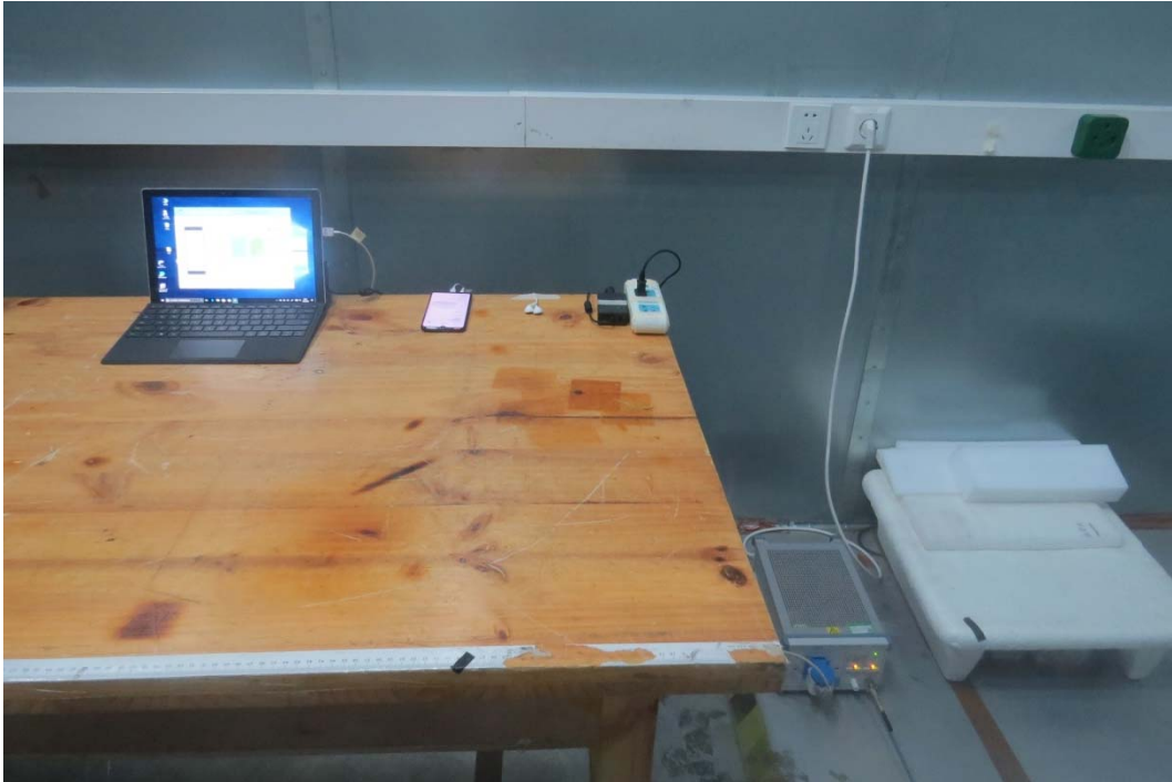
Picture 2 Conducted Emission Test Setup
