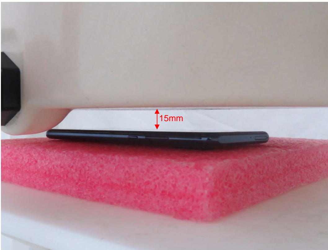
Picture 6: Front Side, the distance from handset to the bottom of the Phantom is 15mm
