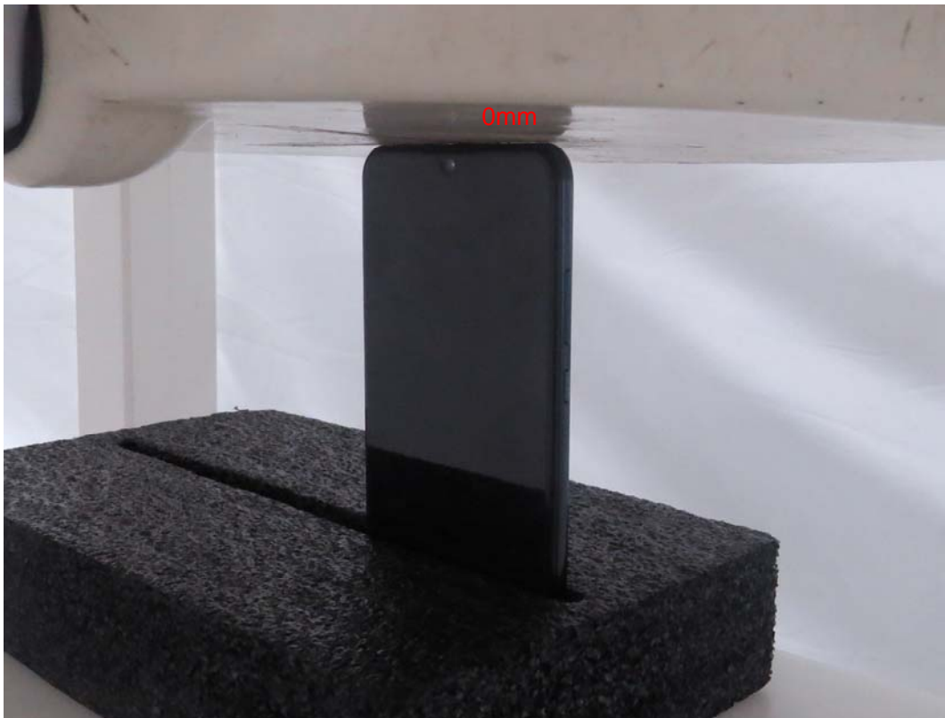
Picture 16: Top Side, the distance from handset to the bottom of the Phantom is 0mm
