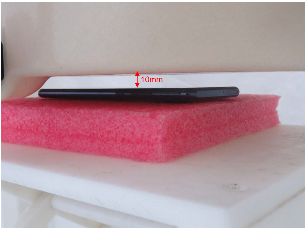
Picture 8: Front Side, the distance from handset to the bottom of the Phantom is 10mm
