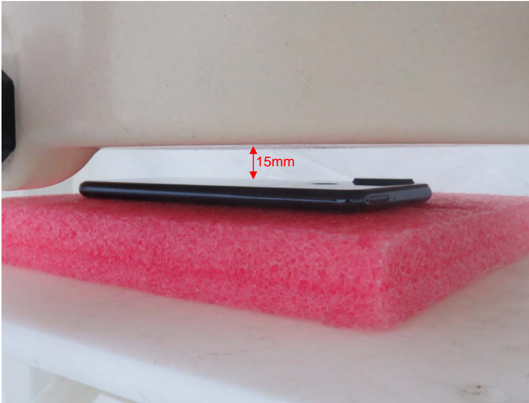
Picture 5: Back Side, the distance from handset to the bottom of the Phantom is 15mm
