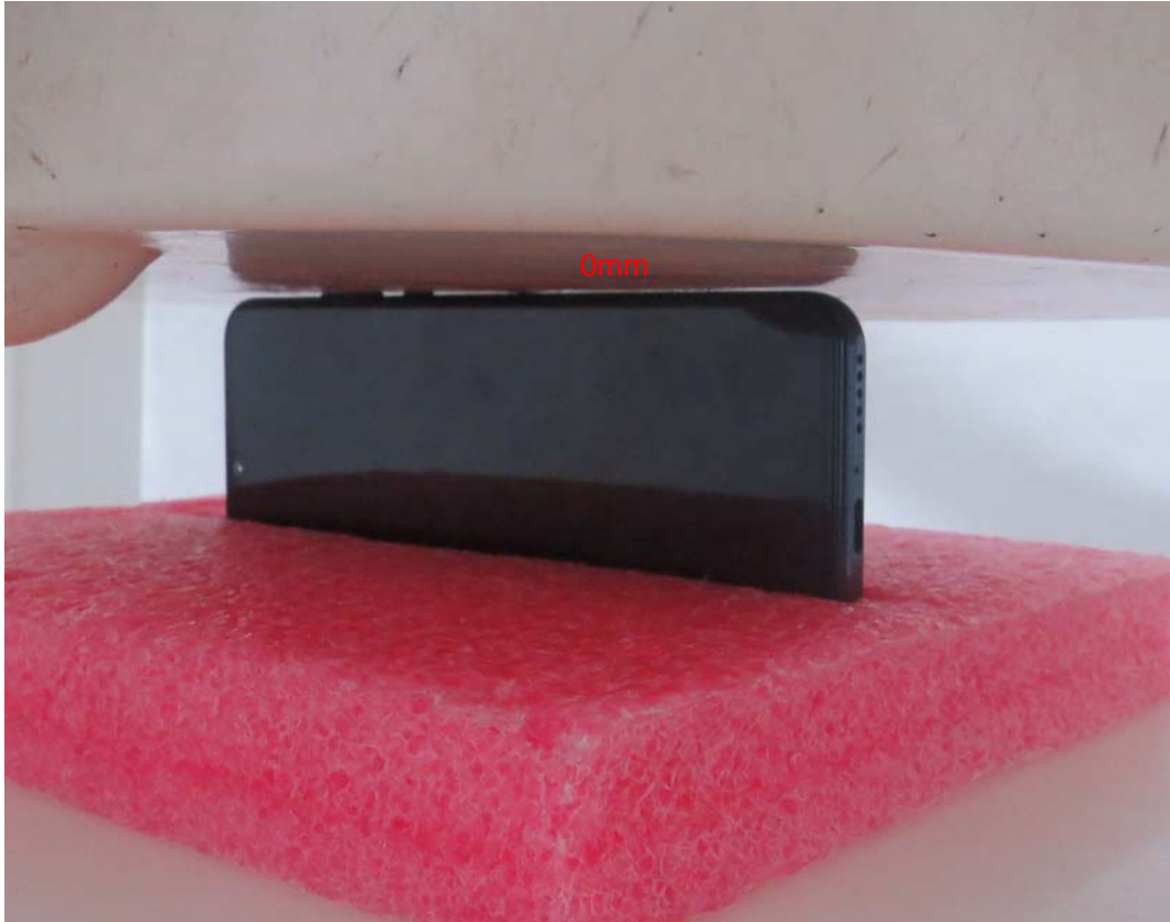
Picture 15: Right Side, the distance from handset to the bottom of the Phantom is 0mm
