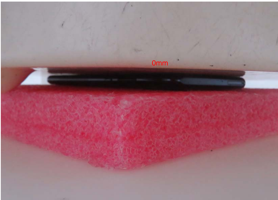
Picture 14: Front Side, the distance from handset to the bottom of the Phantom is 0mm
