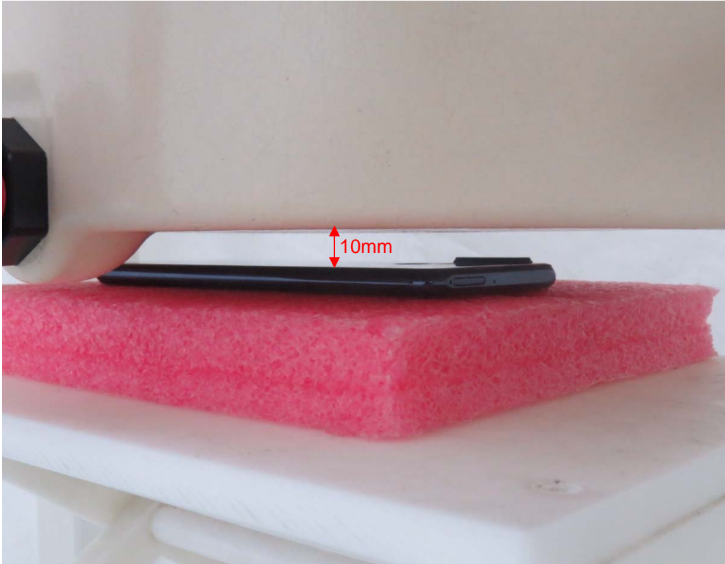
Picture 7: Back Side, the distance from handset to the bottom of the Phantom is 10mm
