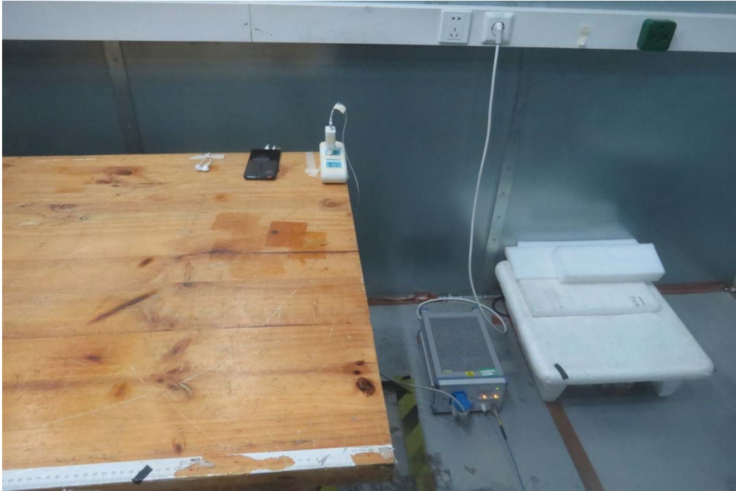
Picture 2 Conducted Emission Test Setup
