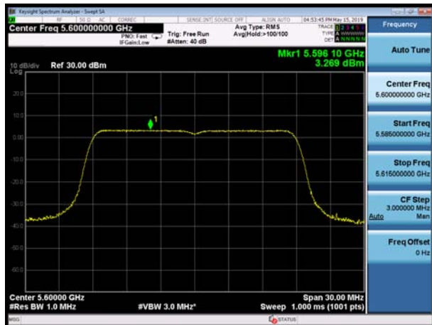
U-NII-2C, 802.11ac VHT20, Channel No.: 140
