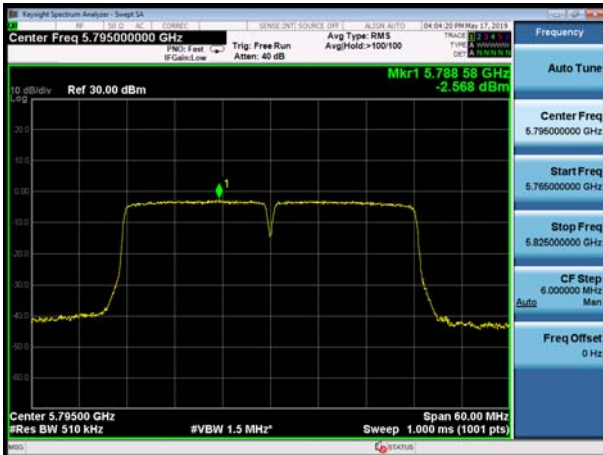
U-NII-3, 802.11ac VHT40, Channel No.: 151
