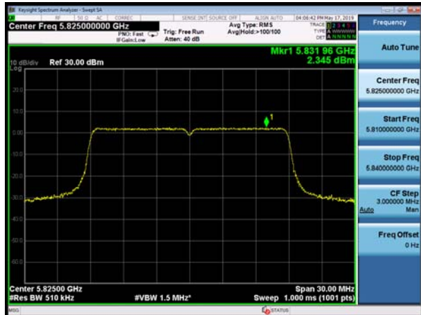
U-NII-3, 802.11ac VHT20, Channel No.: 165
