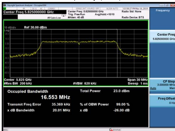
U-NII-3, 802.11a Carrier frequency (MHz): 5825
