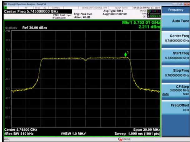
U-NII-3, 802.11ac VHT20, Channel No.: 157
