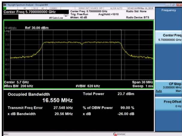
U-NII-2C, 802.11a Carrier frequency (MHz): 5700
