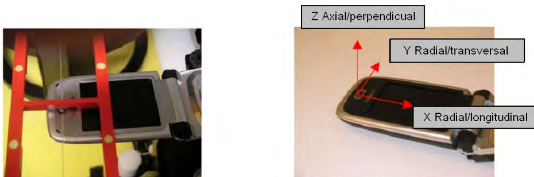
Figure 2. Photo of a typical device positioned under Test Arch and coordinate system
