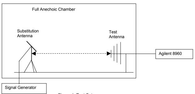
Figure 1. Test Set-up
