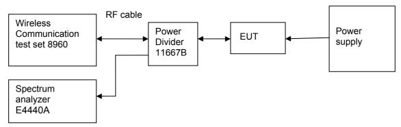
Figure 5. Test Set-up
