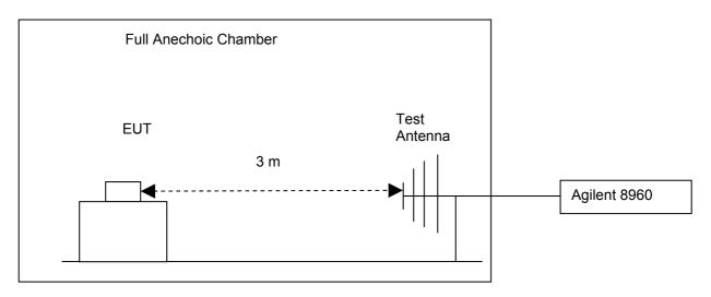
Step 2: Substitution method to verify the maximum ERP
