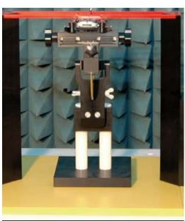
Figure 4 HAC Phantom & Device Holder
