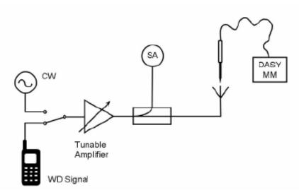
Figure Figure 7 Probe Modulation Factor Test Setup
