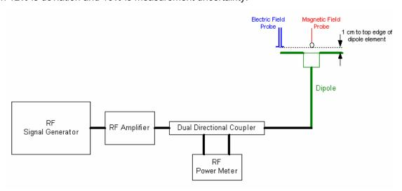
**Figure 6 Dipole Validation Setup**
