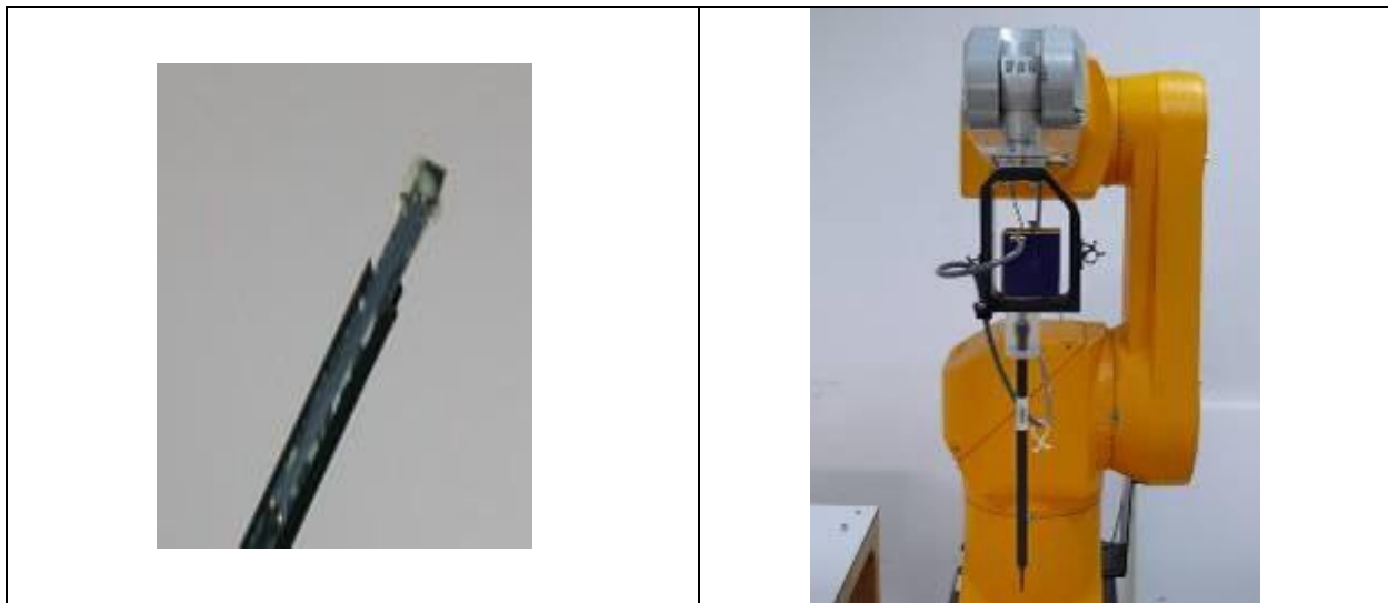
EX3DV4 E-field Probe
