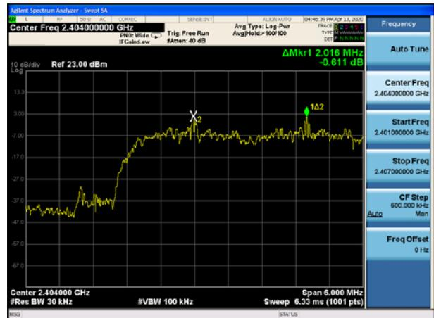
BT 2MHz  $\pi/4$ -DQPSK(4Mbps), Carrier frequency (MHz): 2440
