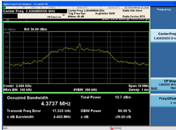
BT 4MHz  $\pi/4$ -DQPSK(8Mbps), Carrier frequency (MHz): 2440
