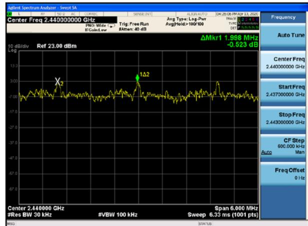
BT 2MHz 8DPSK(6Mbps), Carrier frequency (MHz): 2440
