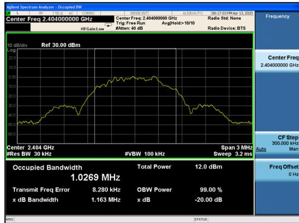
BT UHD BLE 2MHz GFSK(2Mbps), Carrier frequency (MHz): 2404
