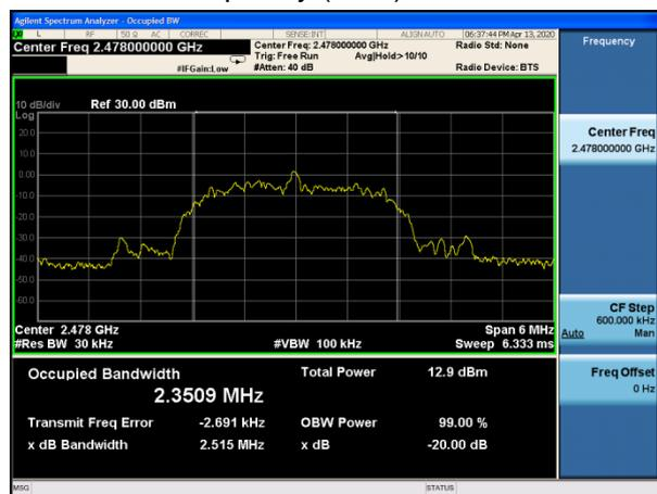
BT 2MHz 8DPSK(6Mbps), Carrier frequency (MHz): 2478
