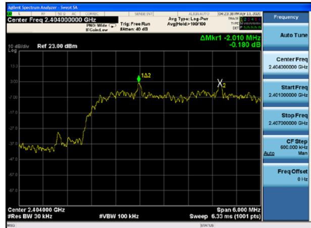
BT 2MHz 8DPSK(6Mbps), Carrier frequency (MHz): 2404
