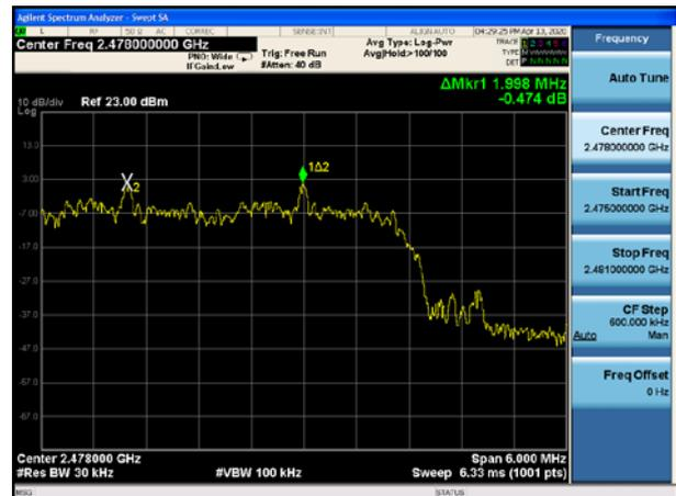
BT 2MHz 8DPSK(6Mbps) CH37, Carrier frequency (MHz): 2478
