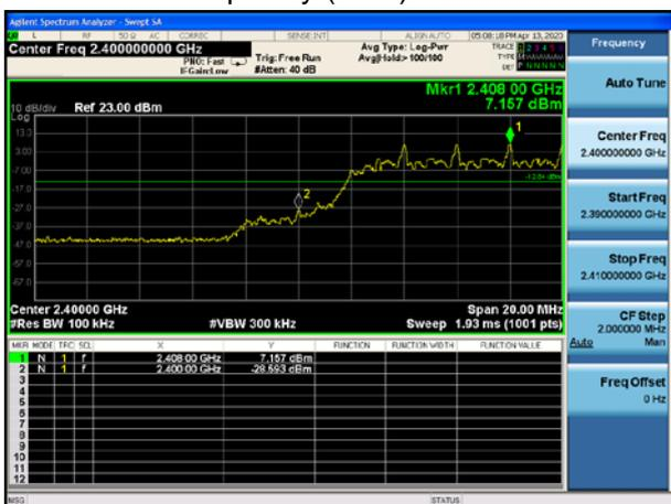
BT UHD 4MHz  $\pi/4$ -DQPSK(8Mbps), Carrier frequency (MHz): 2476
