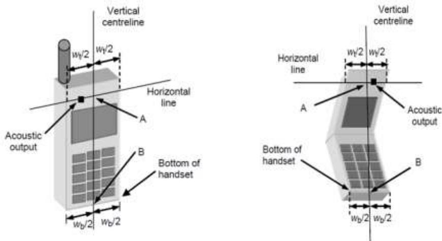
Figure 1 Hand Vertical Center & Horizontal Line Reference Points
