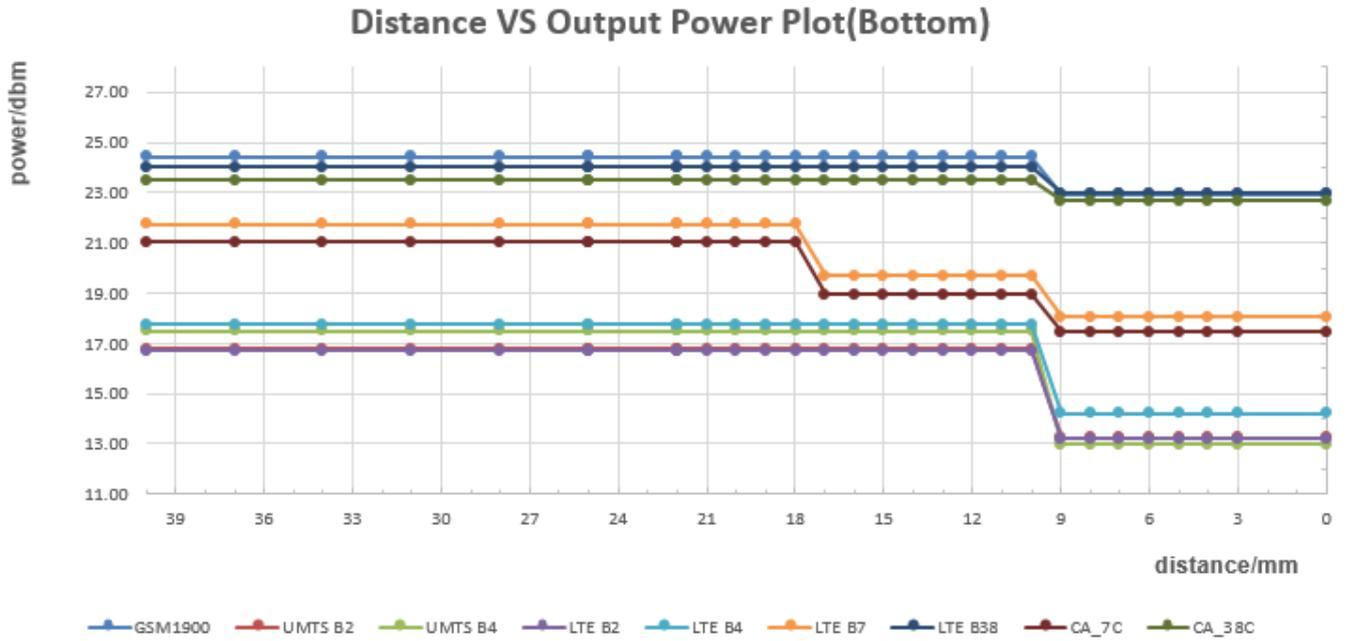
The DUT(Front side) is moved away from the flat phantom(Hotspot on):
