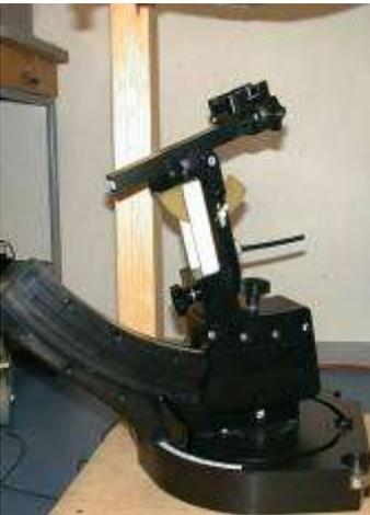
The DASY device holder is constructed of low-loss POM material having the following dielectric parameters: relative permittivity  $\epsilon = 3$  and loss tangent  $\sigma = 0.02$ . The amount of dielectric material has been reduced in the closest vicinity of the device, since measurements have suggested that the influence of the clamp on the test results could thus be lowered.
