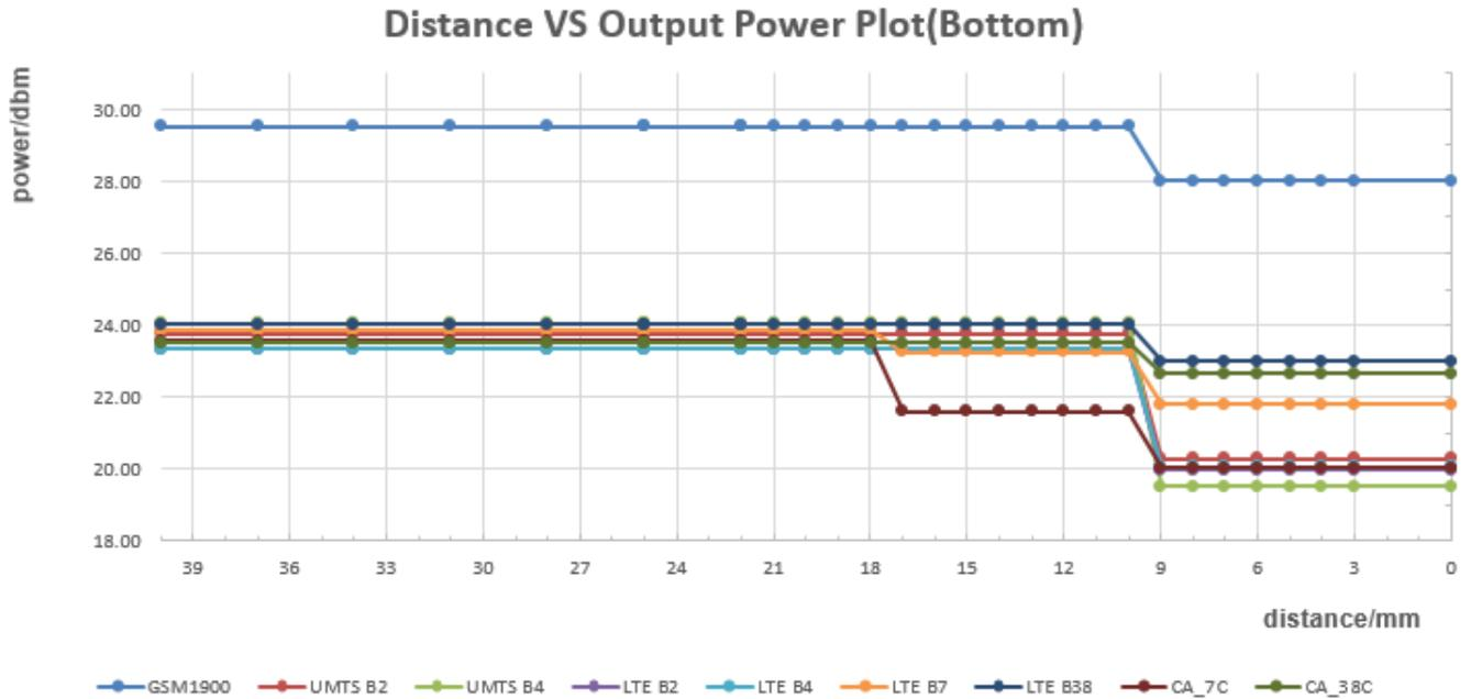
The DUT(Front side) is moved away from the flat phantom(Hotspot off):
