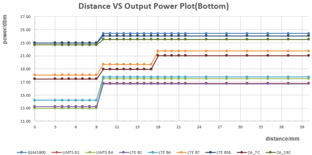
**Conclusion:** It can be ensured that the proximity sensor can be valid triggered for the body exposure condition. (GSM 1900,UMTS Band II/IV,LTE Band 2/4/7/38, UL CA\_7C, UL CA\_38C with Main Antenna)
