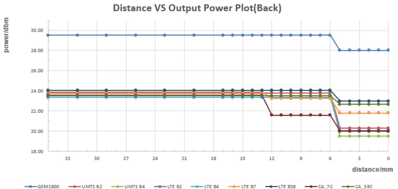
The DUT(Bottom side) is moved towards the flat phantom(Hotspot off):
