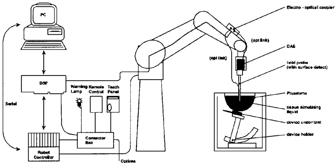
The DAS system for performing compliance tests consists of the following items:
