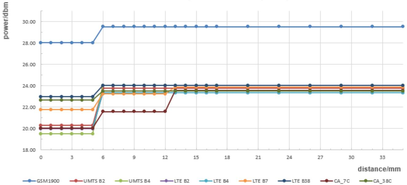
The DUT(Bottom side) is moved away from the flat phantom(Hotspot off):
