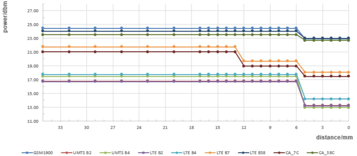
The DUT(Bottom side) is moved towards the flat phantom(Hotspot on):
