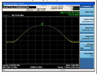
BT UHD BLE 2MHZ GFSK(2Mbps), Carrier frequency (MHz): 2404
