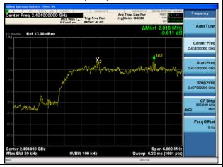
BT 2MHZ 8DPSK(6Mbps), Carrier frequency (MHz): 2440
