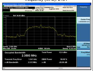
BT 2MHZ 8DPSK(6Mbps), Carrier frequency (MHz): 2404
