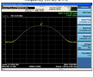
BT UHD BLE 2MHZ GFSK(2Mbps), Carrier frequency (MHz): 2478
