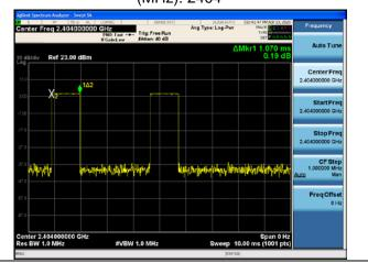
BT UHD BLE 2MHZ GFSK(1Mbps), Carrier frequency (MHz): 2440
