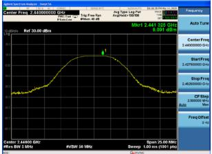
BT 4MHz π/4-DQPSK(8Mbps), Carrier frequency (MHz): 2476
