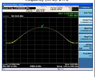
BT 2MHZ 8DPSK(6Mbps), Carrier frequency (MHz): 2478
