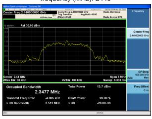
BT 2MHZ 8DPSK(6Mbps), Carrier frequency (MHz): 2440
