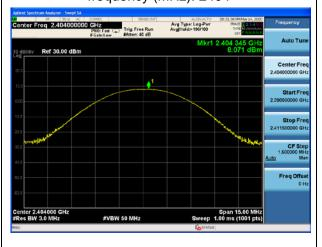
BT 2MHZ 8DPSK(6Mbps), Carrier frequency (MHz): 2404
