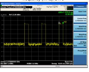
BT 2MHZ 8DPSK(6Mbps) CH37, Carrier frequency (MHz): 2478
