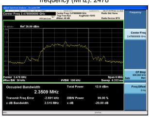
BT 2MHZ 8DPSK(6Mbps), Carrier frequency (MHz): 2478
