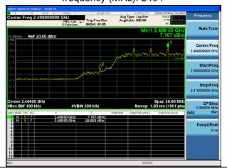
BT UHD 4MHz π/4-DQPSK(8Mbps), Carrier frequency (MHz): 2476
