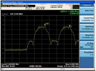
BT UHD BLE 2MHZ GFSK(1Mbps), Carrier frequency (MHz): 2440
