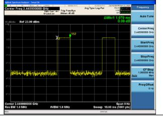
BT UHD BLE 2MHZ GFSK(1Mbps), Carrier frequency (MHz): 2478
