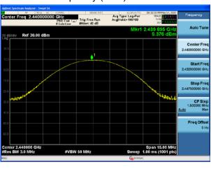
BT 2MHZ 8DPSK(6Mbps), Carrier frequency (MHz): 2440
