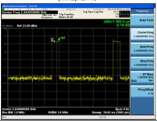
BT 2MHZ 8DPSK(6Mbps), Carrier frequency (MHz): 2440
