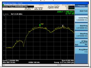
BT UHD BLE 2MHZ GFSK(2Mbps), Carrier frequency (MHz): 2440
