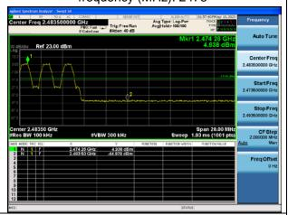
BT UHD BLE 2MHZ GFSK(2Mbps), Carrier frequency (MHz): 2478
