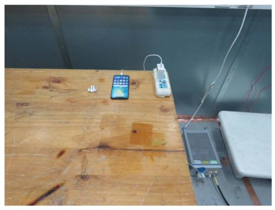
Picture 2 Conducted Emission Test Setup
