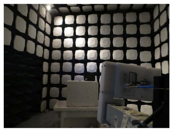
18GHz - 26.5GHz Picture 1 Radiated Emission Test Setup
