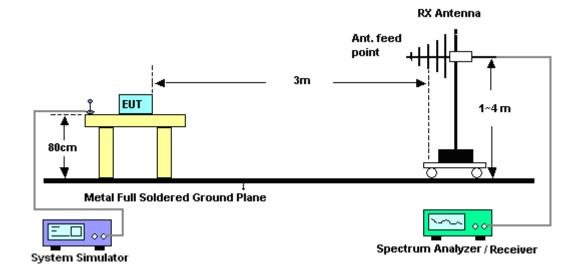
For radiated test above 1GHz
