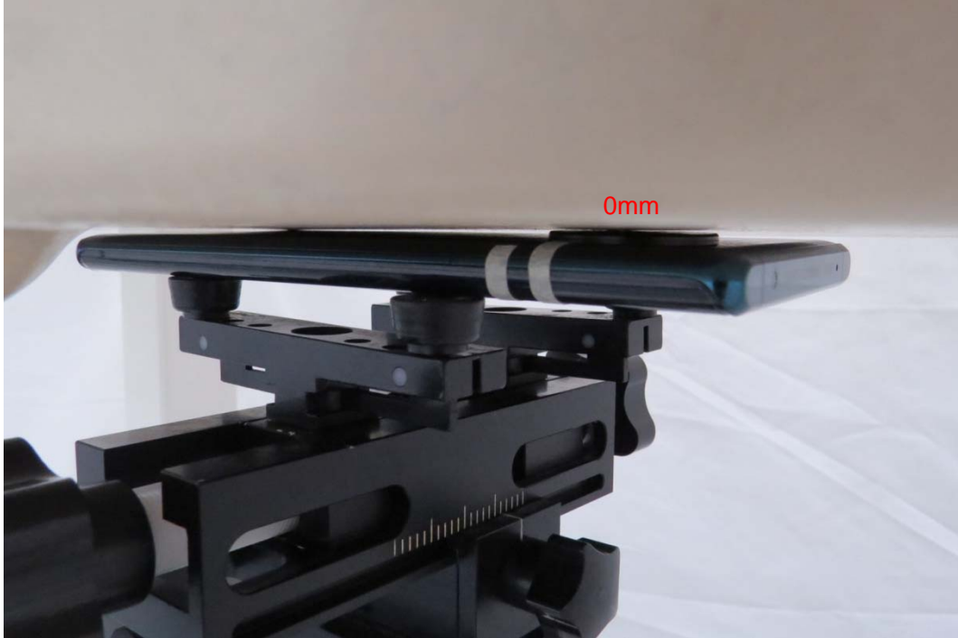
Picture 25: Back Side, the distance from handset to the bottom of the Phantom is 0mm
