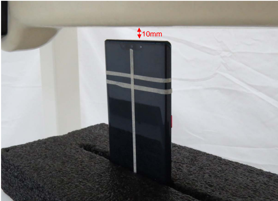
Picture 19: Top Side, the distance from handset to the bottom of the Phantom is 10mm
