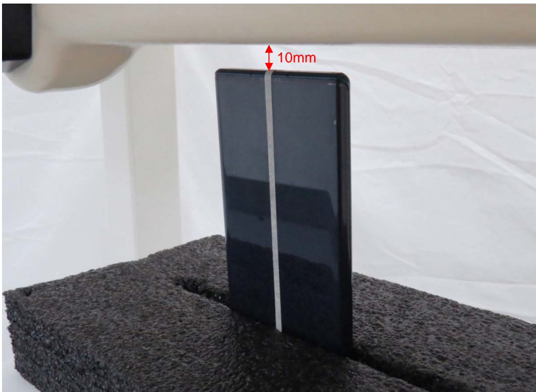
Picture 20: Bottom Side, the distance from handset to the bottom of the Phantom is 10mm
