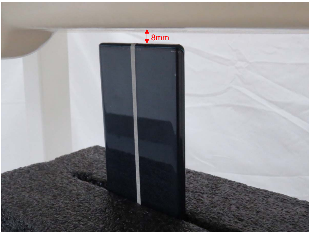
Picture 24: Bottom Side, the distance from handset to the bottom of the Phantom is 8mm
