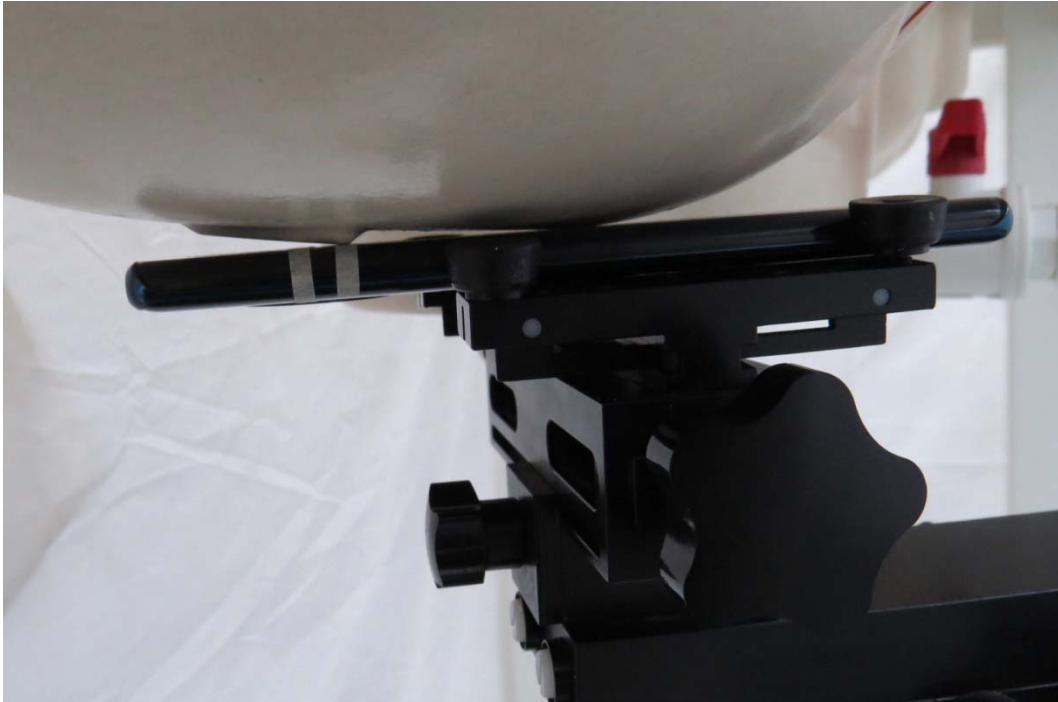
Picture 7: Right Hand Touch Cheek Position (the best acoustic position)
