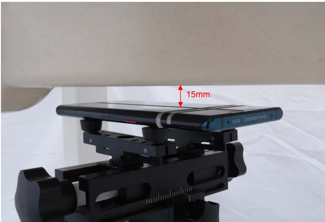
Picture 14: Front Side, the distance from handset to the bottom of the Phantom is 15mm
