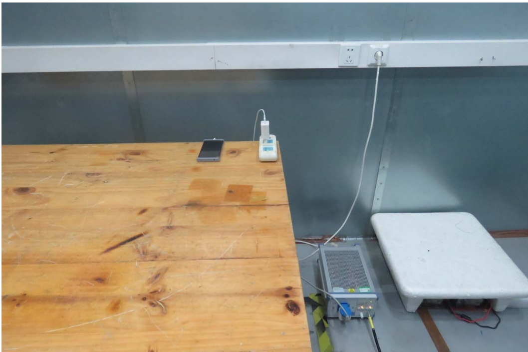
Picture 2 Conducted Emission Test Setup
