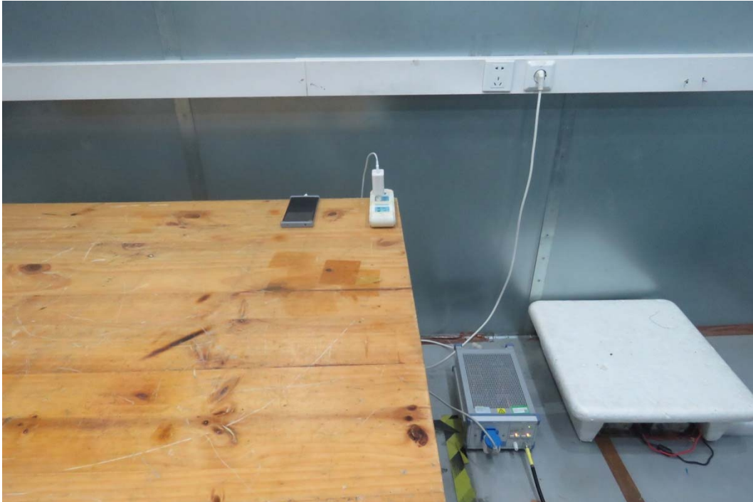
Picture 2 Conducted Emission Test Setup
