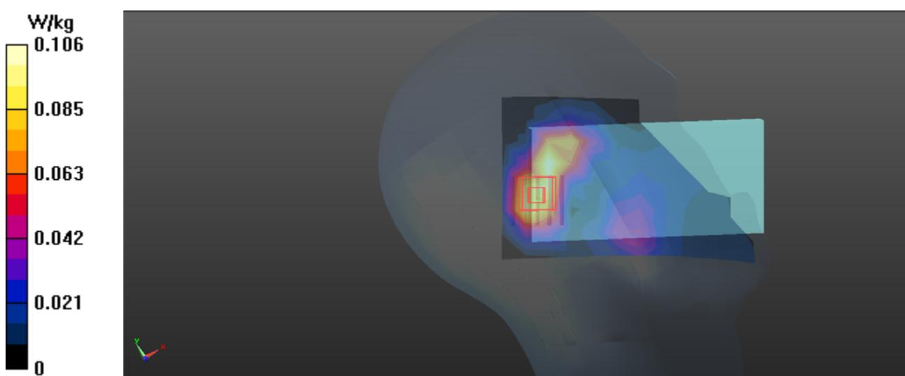
**P57 LTE B4\_QPSK20M\_1RB Offset 50\_Right Cheek\_Ch20300\_SIM1\_Battery3****DUT: 1801C011;**
