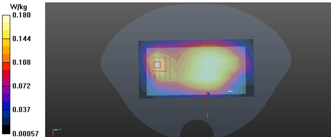
**P391 LTE B7\_QPSK20M\_1RB Offset 50\_Rear Face\_Ch21100\_1.5cm\_Sensor off\_SIM1\_Battery3****DUT: 1801C011;**
