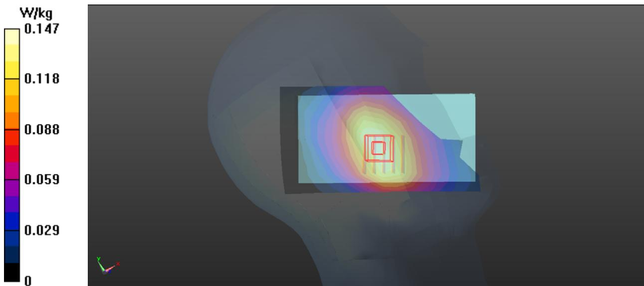
**P46 LTE B2\_QPSK20M\_1RB Offset 50\_Left Tilted\_Ch18700\_SIM1\_Battery3****DUT: 1801C011;**
