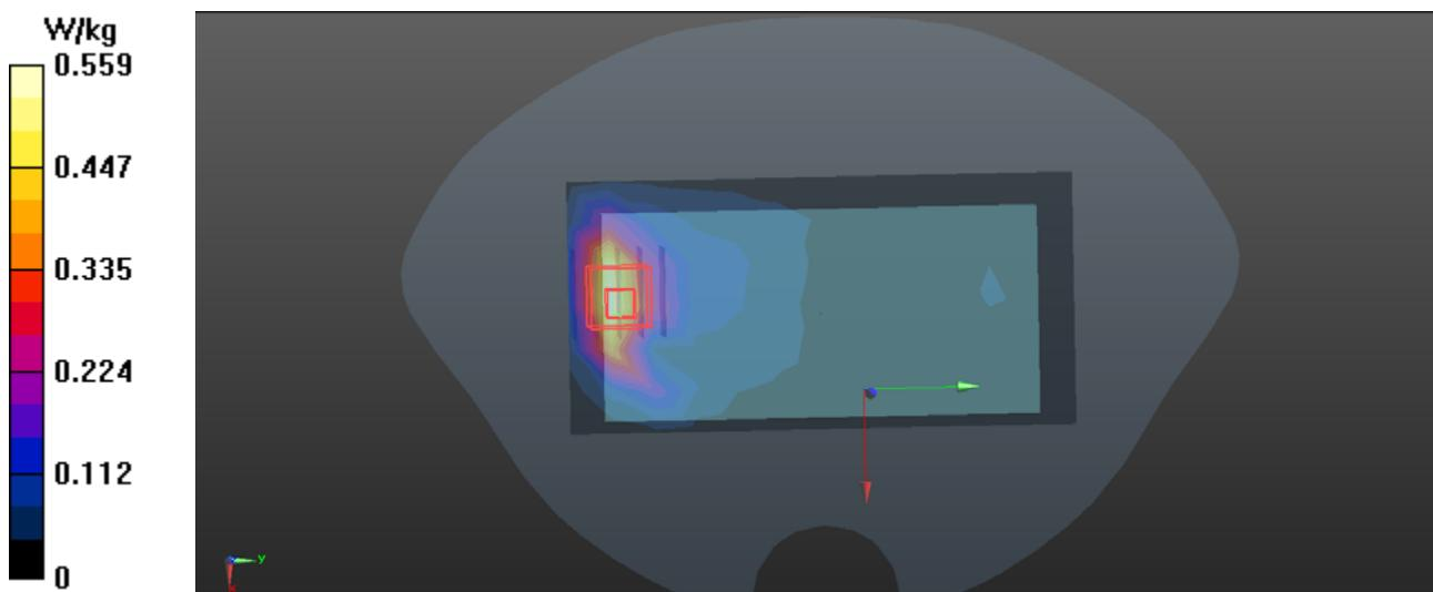
**P361 LTE B4\_QPSK20M\_1RB Offset 50\_Bottom Side\_Ch20300\_1.1cm\_Sensor off\_SIM1\_Battery2\_Extremity****DUT: 1801C011;**
