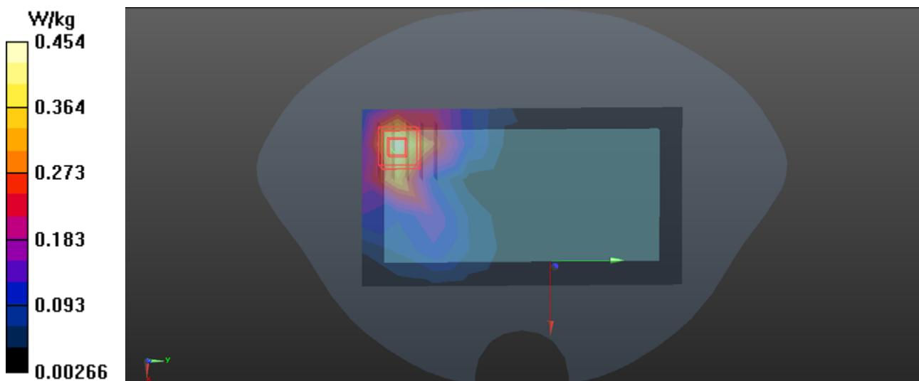
**P407 LTE B7\_QPSK20M\_1RB Offset 50\_Rear Face\_Ch21100\_1cm\_Sensor off\_SIM1\_Battery3****DUT: 1801C011;**
