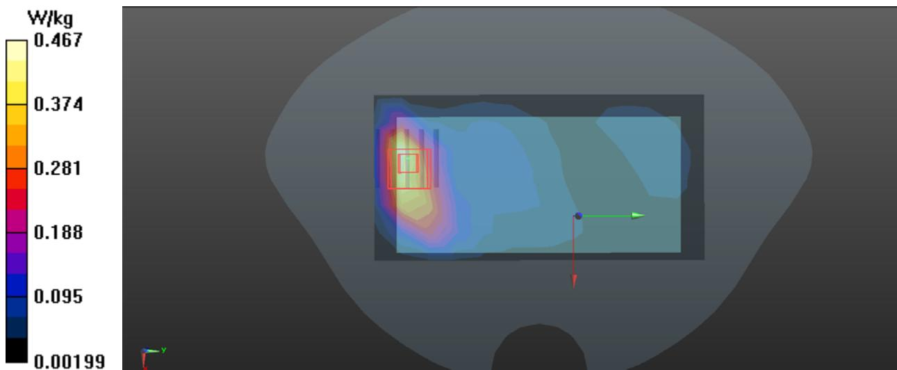
**P259 UMTS B4\_RMC12.2k\_Rear Face\_Ch1413\_1.5cm\_Sensor off\_SIM2\_Battery1****DUT: 1801C011;**
