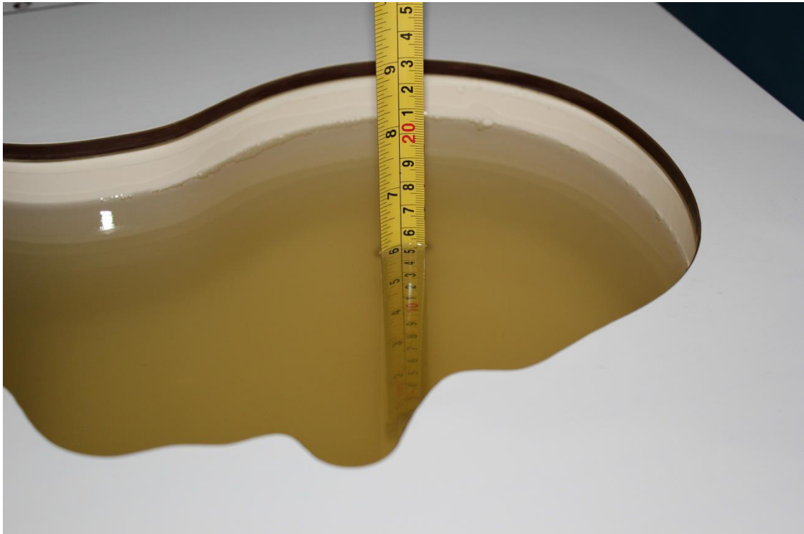
Picture 7-7: Liquid depth in the Head Phantom(2550MHz)
