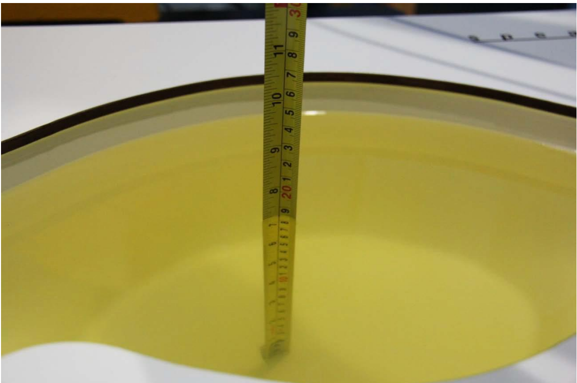
Picture 7-6: Liquid depth in the Flat Phantom(2450MHz)
