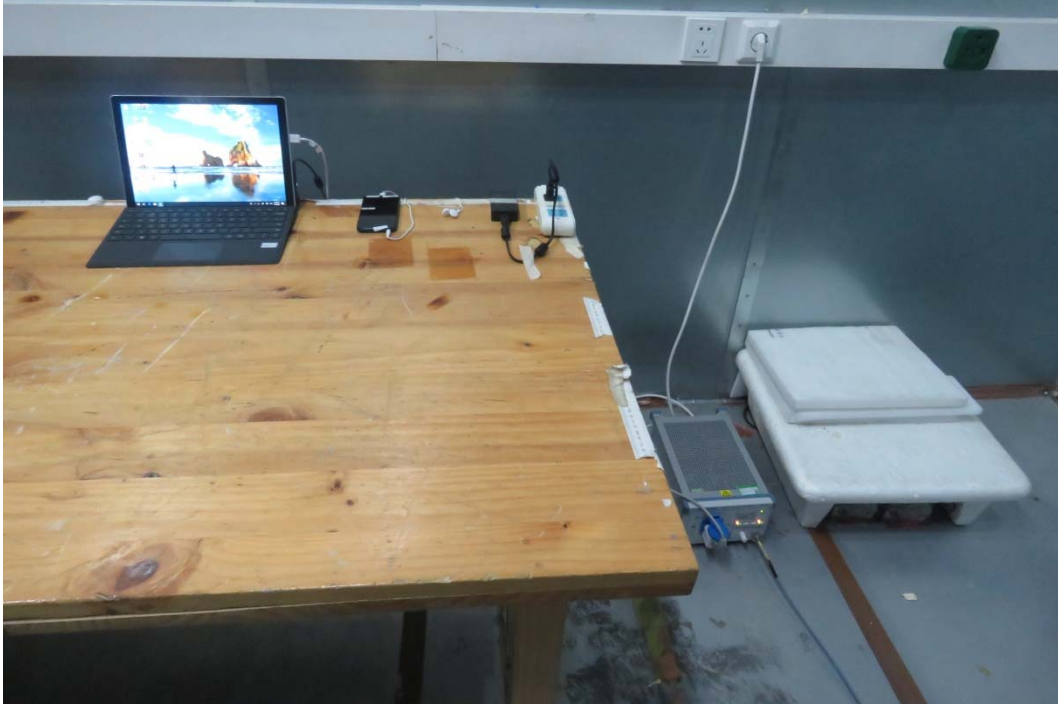
Picture 2 Conducted Emission Test Setup
