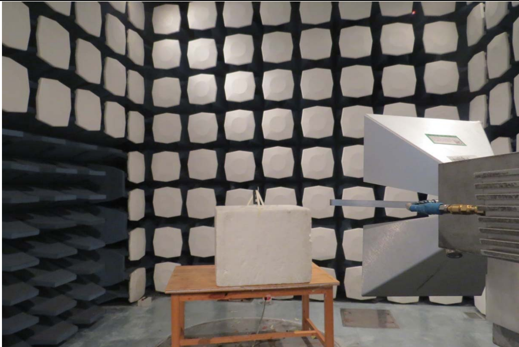
Picture 1: Radiated Spurious Emissions Test setup
