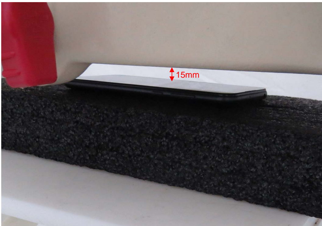
Picture 6: Front Side, the distance from handset to the bottom of the Phantom is 15mm
