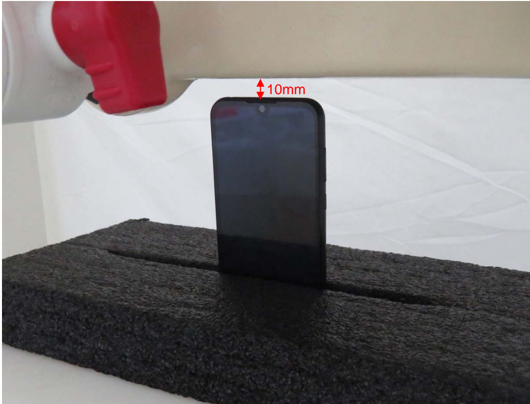
Picture 11: Top Side, the distance from handset to the bottom of the Phantom is 10mm
