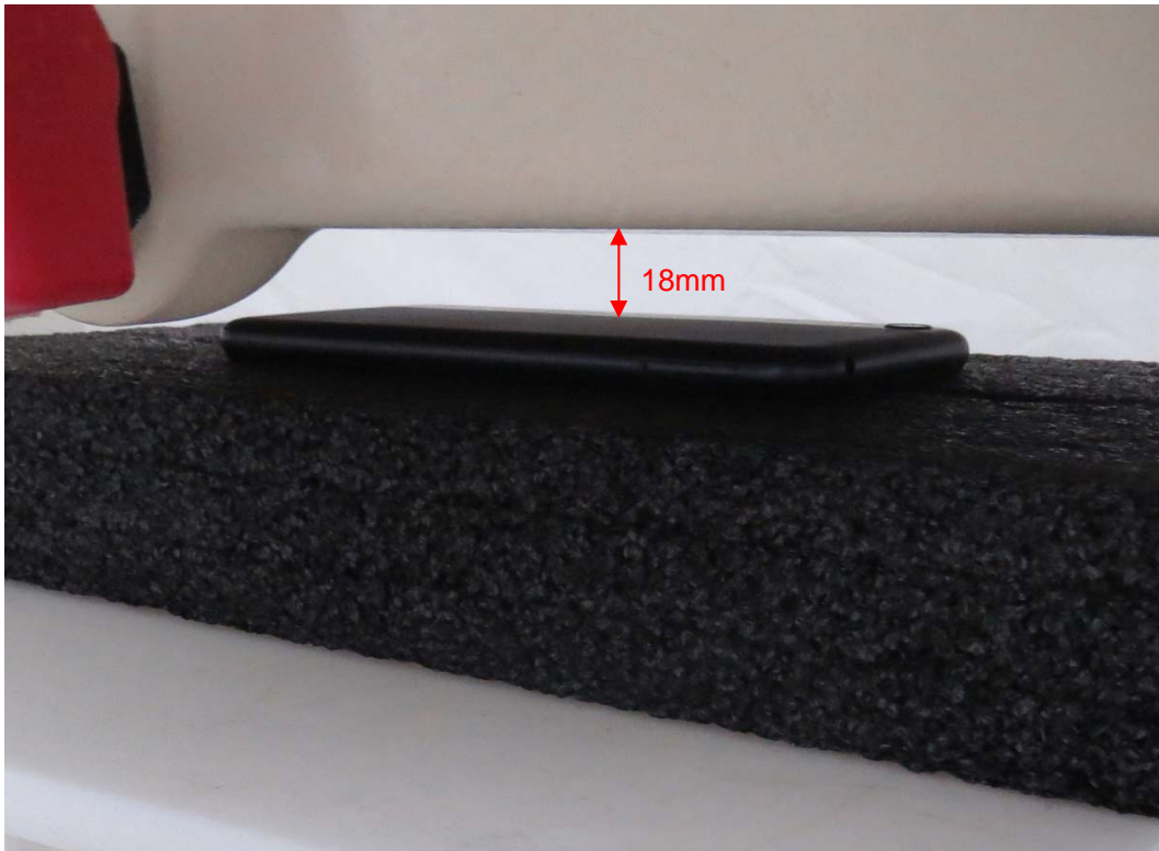
Picture 5: Back Side, the distance from handset to the bottom of the Phantom is 18mm
