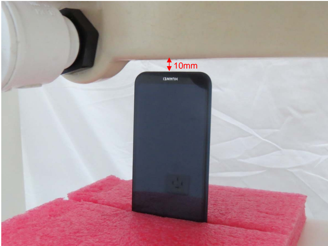
Picture 13: Bottom Edge, the distance from handset to the bottom of the Phantom is 10mm
