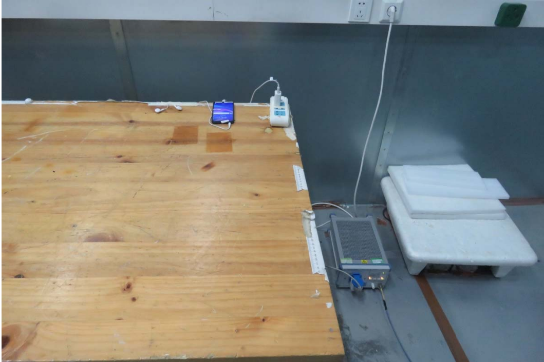
Picture 2 Conducted Emission Test Setup
