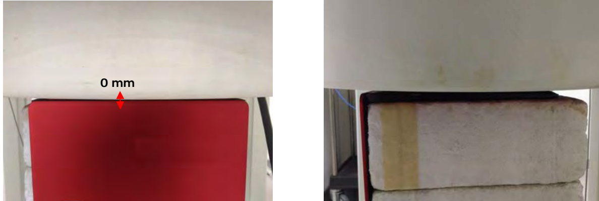
Fig.3 EUT Bottom side to flat phantom
