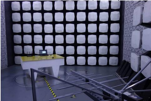
1.3 Radiated Emissions (Above 1GHz) Test Setup
