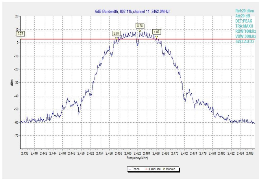
Fig.12 Occupied 6dB Bandwidth (802.11b, Ch 11)
