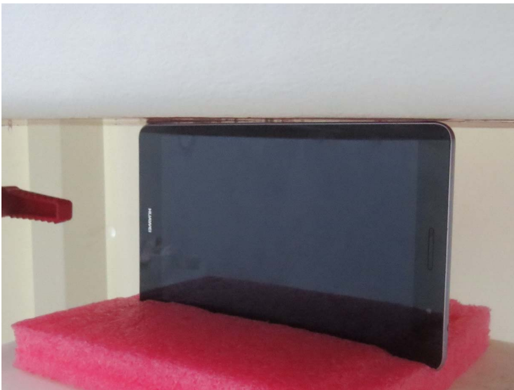
Picture 2: Left Side, the distance from handset to the bottom of the Phantom is 0mm
