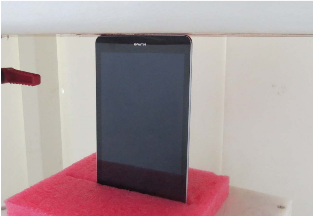
Picture 5: Bottom Side, the distance from handset to the bottom of the Phantom is 0mm
