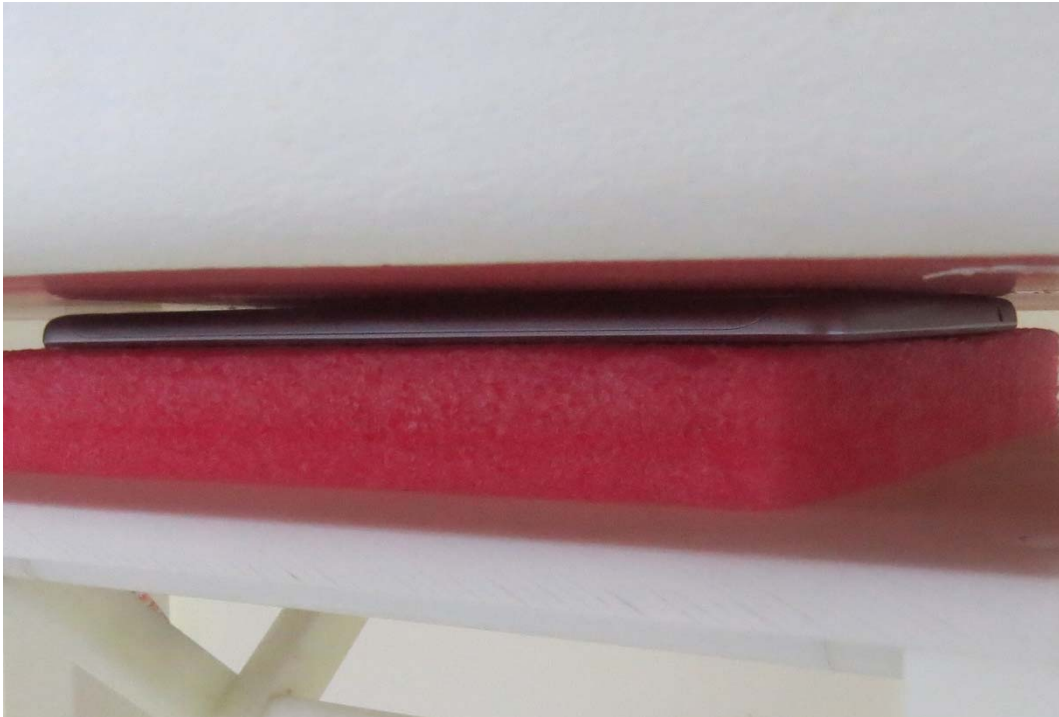
Picture 1: Back Side, the distance from handset to the bottom of the Phantom is 0mm
