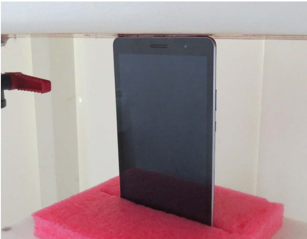
Picture 4: Top Side, the distance from handset to the bottom of the Phantom is 0mm
