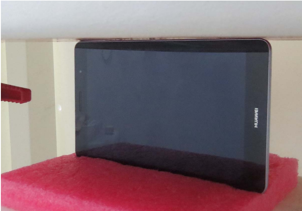
Picture 3: Right Side, the distance from handset to the bottom of the Phantom is 0mm
