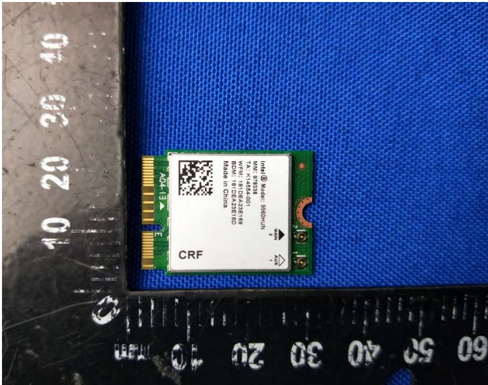
RF Module TOP VIEW (WITH SHIELDING)
