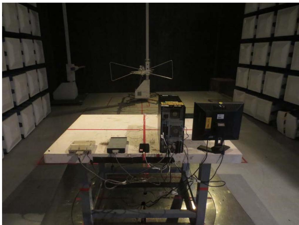
**Radiated Measurement Photos – 30MHz to 1GHz****Mode 2-6**
