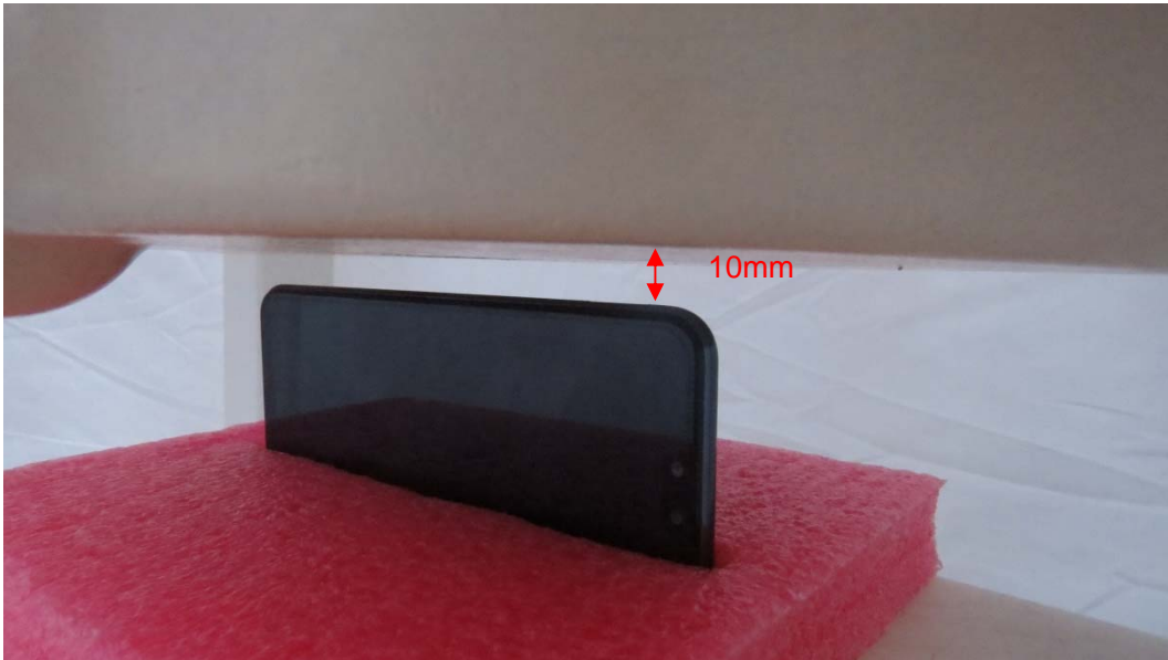
Picture 9: Left Edge, the distance from handset to the bottom of the Phantom is 10mm
