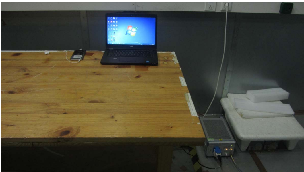
Picture 2 Conducted Emission Test Setup
