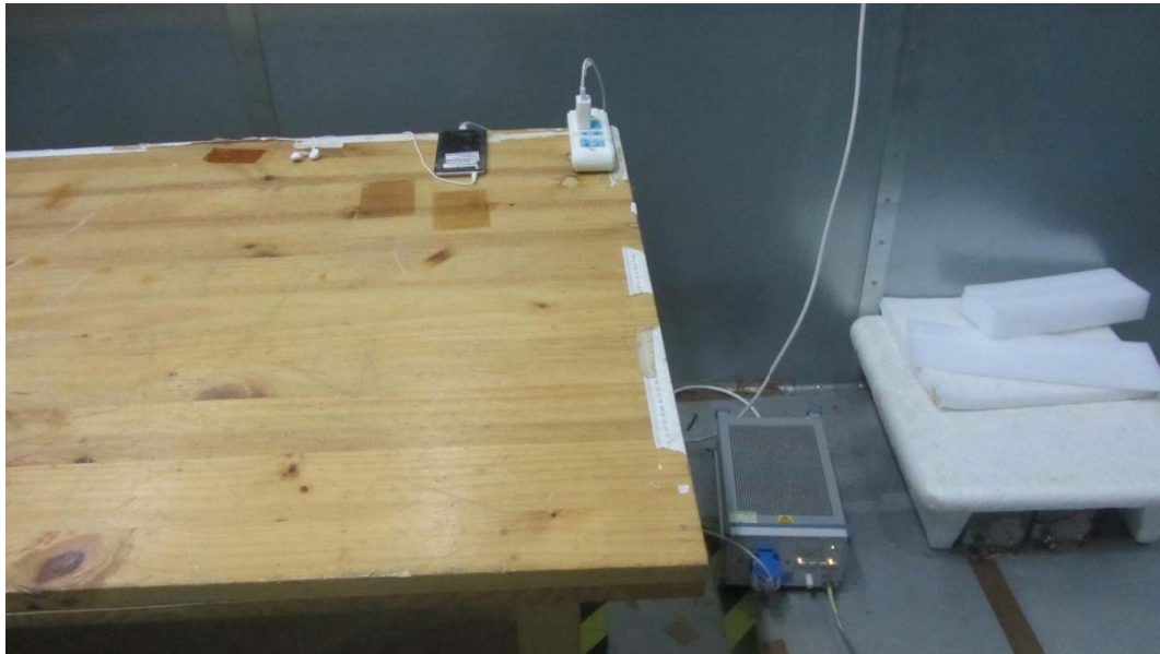
Picture 3 Conducted Emission Test Setup
