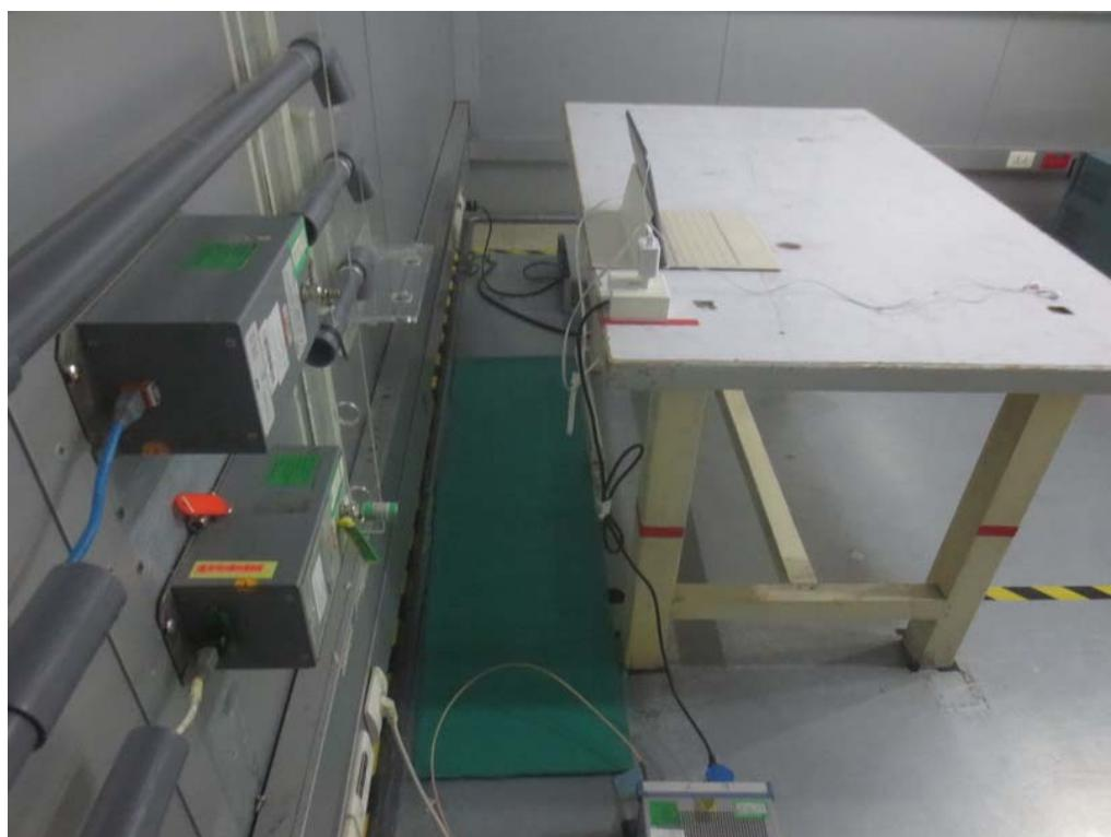
**Radiated emission below 1 GHz test photos****Mode 1 ~ Mode 7**
