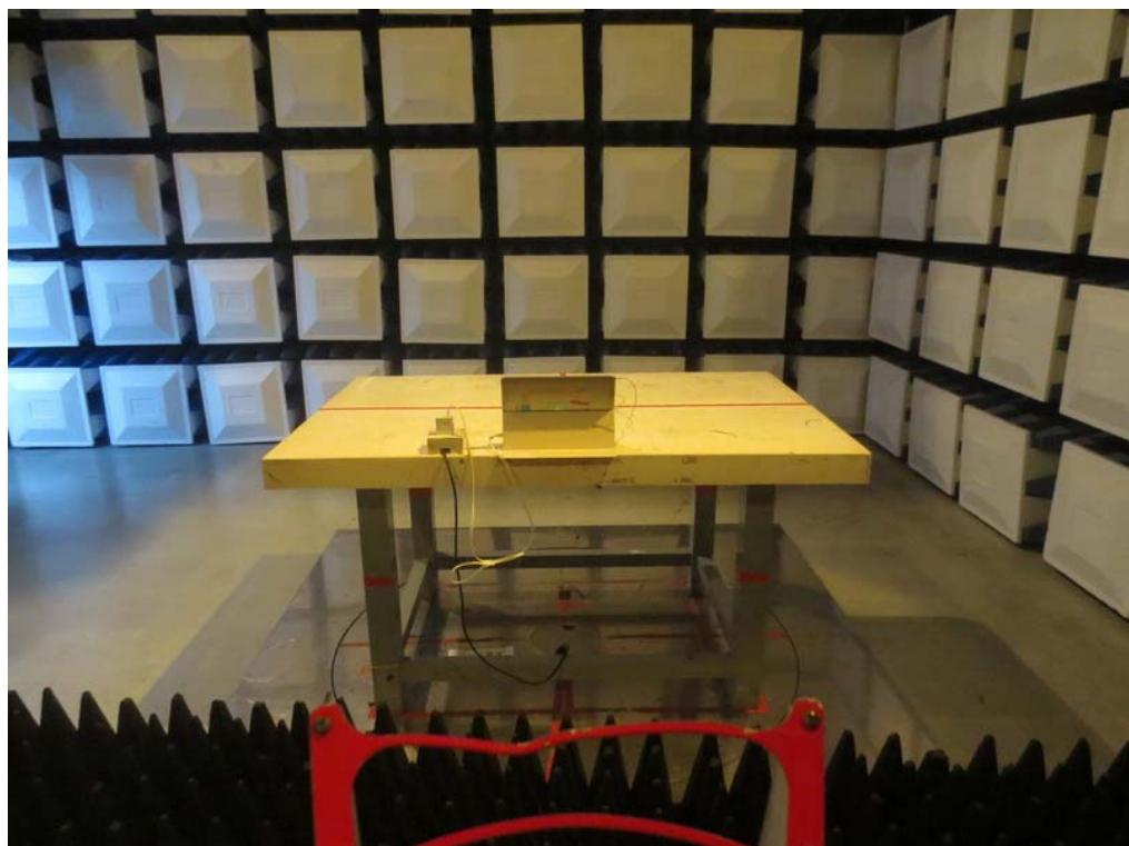
**Radiated emission above 1 GHz test photos****Mode 8**
