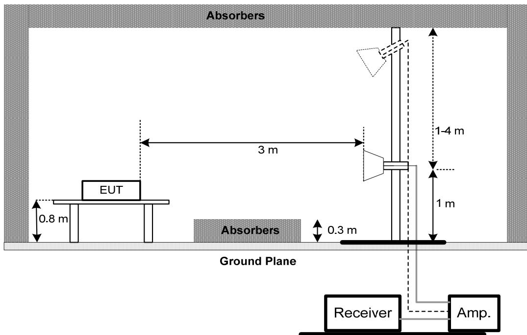
(C) Radiated Emission Test Set-Up Frequency 18 GHz-40GHz
