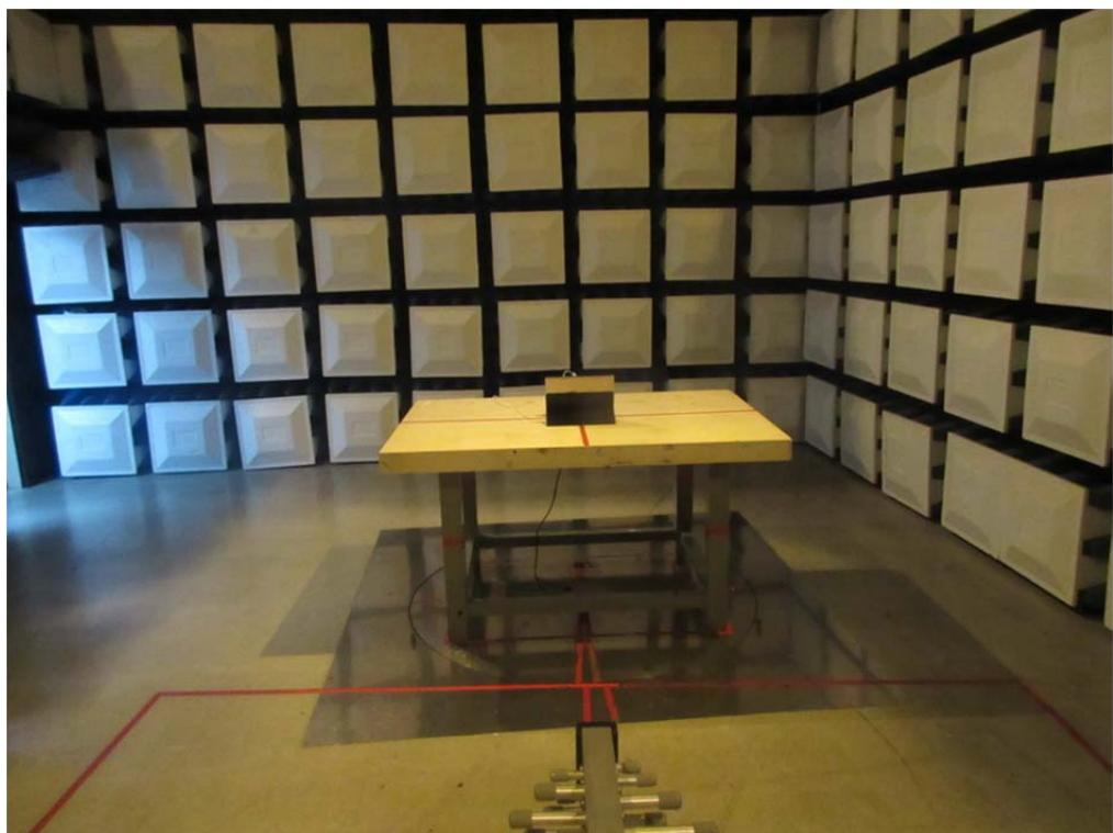
**30MHz to 1000MHz Radiated Measurement Photos****Adapter: SALCOMP**
