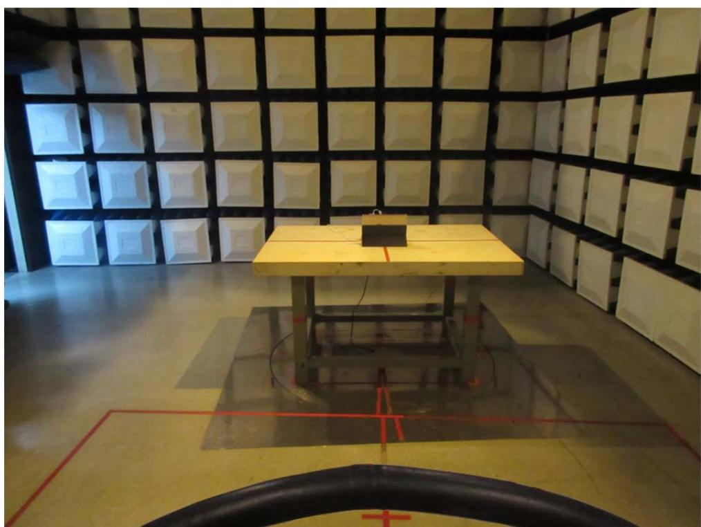
**30MHz to 1000MHz Radiated Measurement Photos****Adapter: BYD**
