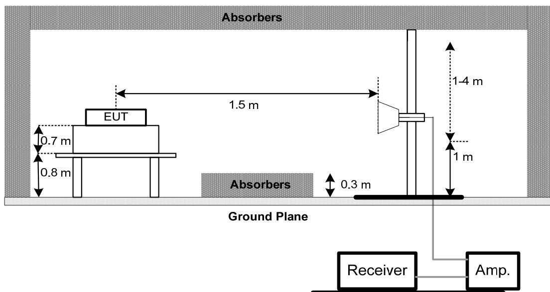
(C) For Radiated Emissions Below 30MHz
