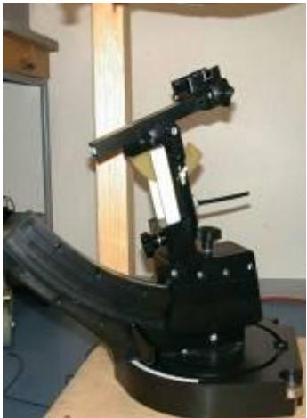
The DASY device holder is constructed of low-loss POM material having the following dielectric parameters: relative permittivity  $\epsilon = 3$  and loss tangent  $\sigma = 0.02$ . The amount of dielectric material has been reduced in the closest vicinity of the device, since measurements have suggested that the influence of the clamp on the test results could thus be lowered. The device holder permits the device to be positioned with a tolerance of  $\pm 1^\circ$  in the tilt angle.
