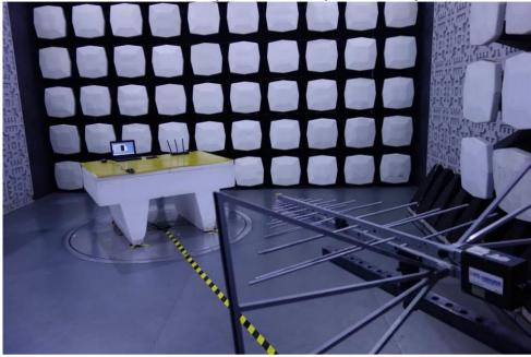
1.3 Radiated Emissions (Above 1GHz) Test Setup
