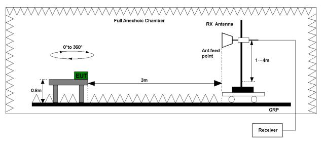
Figure 2. Test set-up of radiated disturbance (above 1GHz)
