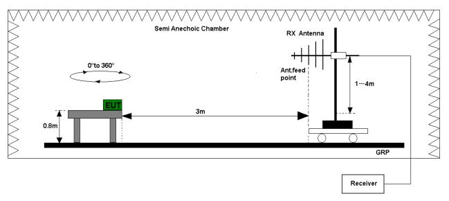
Figure 1.Test set-up of radiated disturbance(30MHz-1GHz)
