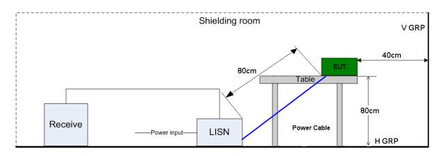
Figure 3. Test Set-up of conducted disturbance
