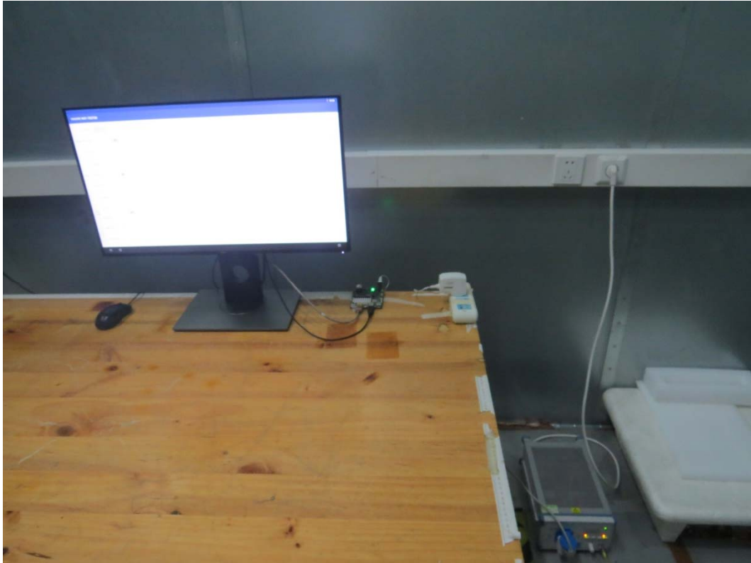
Picture 3 Conducted Emission Test Setup
