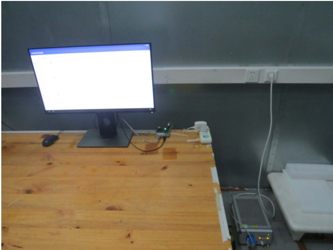
Picture 2 Conducted Emission Test Setup
