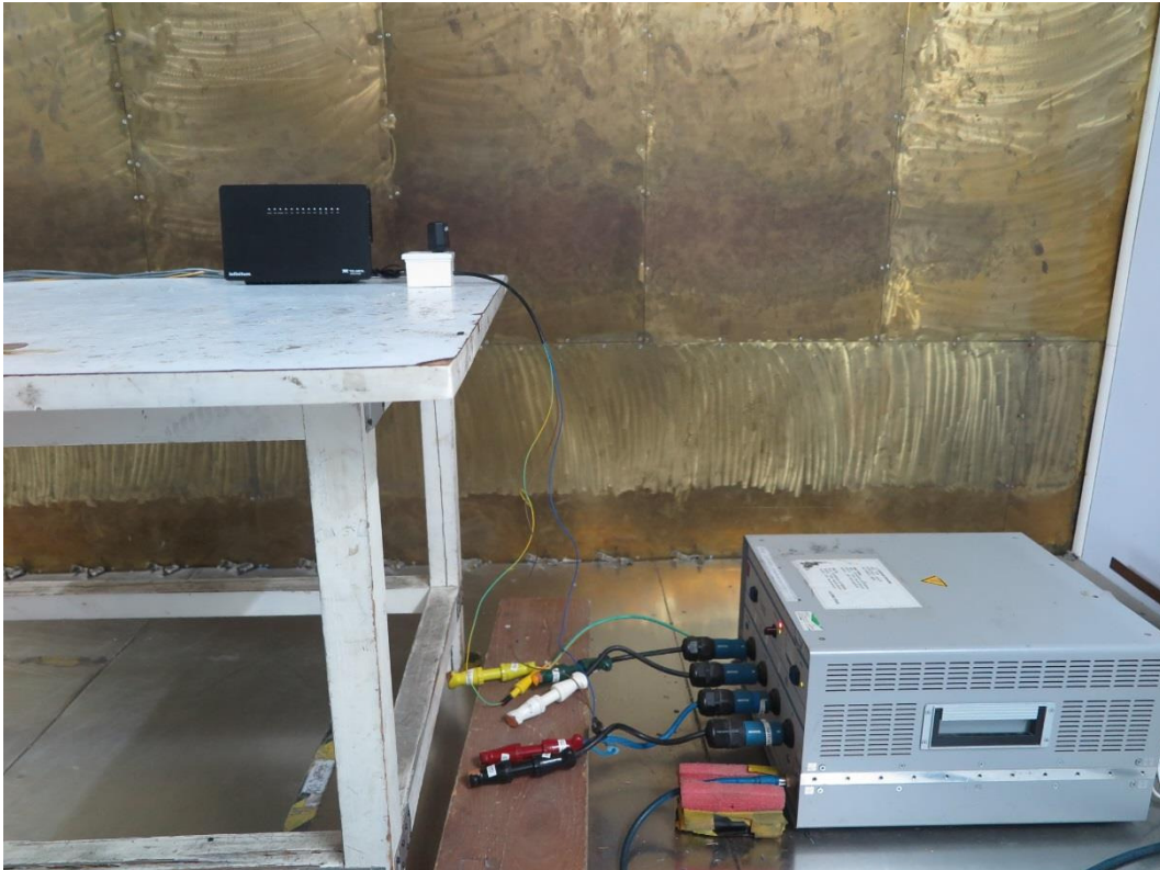
Conducted emissions of AC power port
