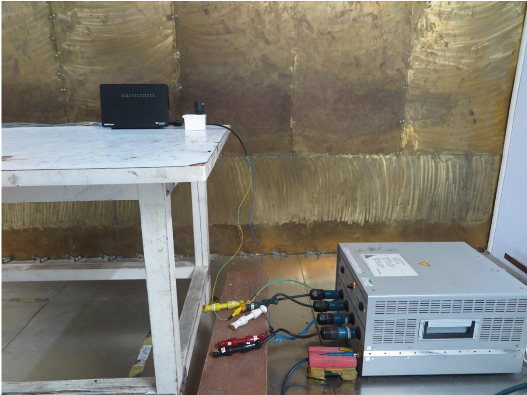
Conducted emissions of AC power port
