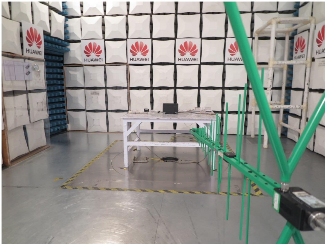
Radiated emission for 30 MHz-1 GHz
