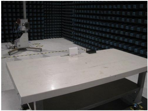
Test Mode : Transmitting Description : Back View of Radiated Emission Test Setup for 1~18GHz
