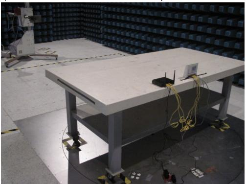
Test Mode : Transmitting Description : Front View of Radiated Emission Test Setup for Above 18GHz
