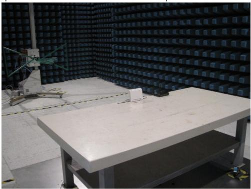
Test Mode : Transmitting Description : Back View of Radiated Emission Test Setup for Below 1GHz
