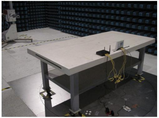
Test Mode : Transmitting Description : Back View of Radiated Emission Test Setup for Above 18GHz
